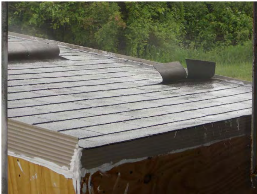
Photo No. 6 Roof System During 110 MPH Phase
