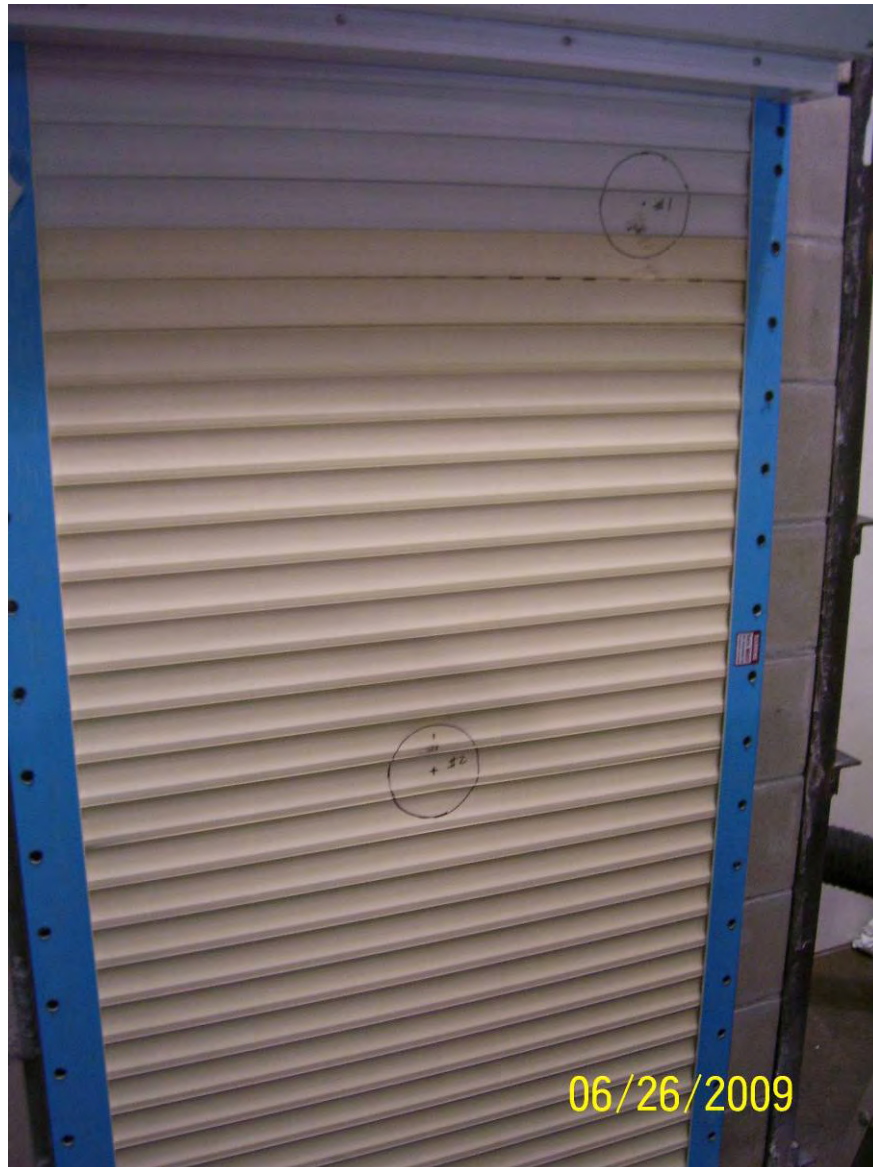
Photo No. 4 Impact Specimen #3 No penetrations or openings
