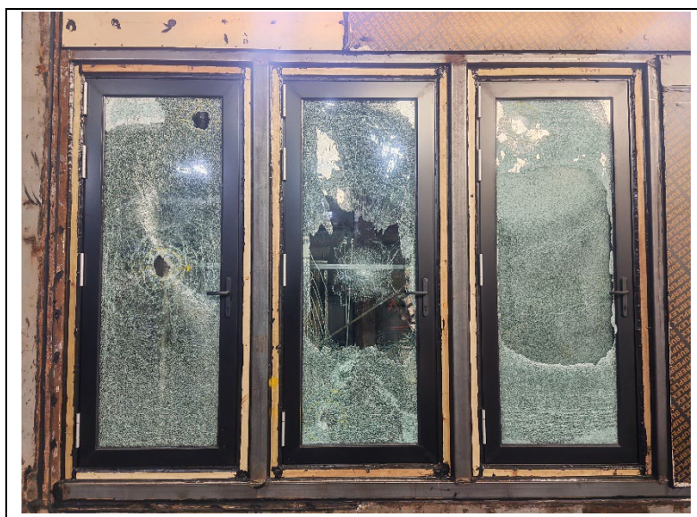
Photo No. 2 Specimens #01, #02 and #03 after impact test (Testing on December 1, 2025)
