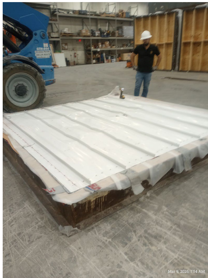
Photo No. 1 Aluminum Deck After Testing
