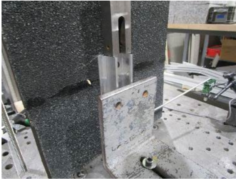
Photo No. 3 Shear Parallel to the Track
