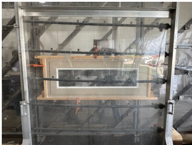
Photo No. 1 Water test setup
