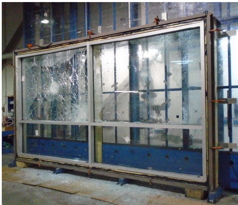
Photo No. 4 Test Specimen #1 during cyclic loading
