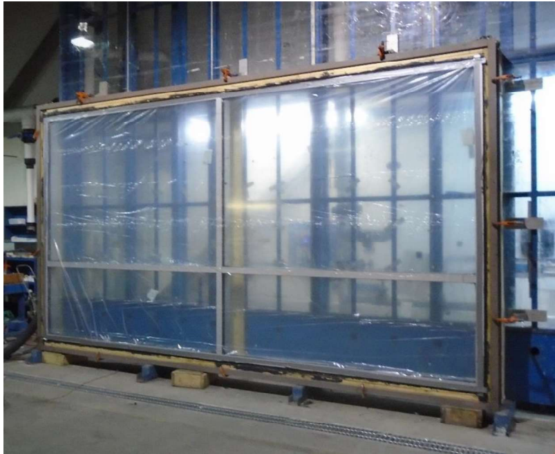
Photo No. 1 Test Specimen #1 during air infiltration
