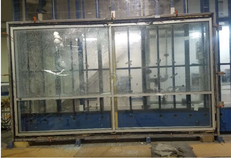
Photo No. 5 Test Specimen #2 during cyclic loading
