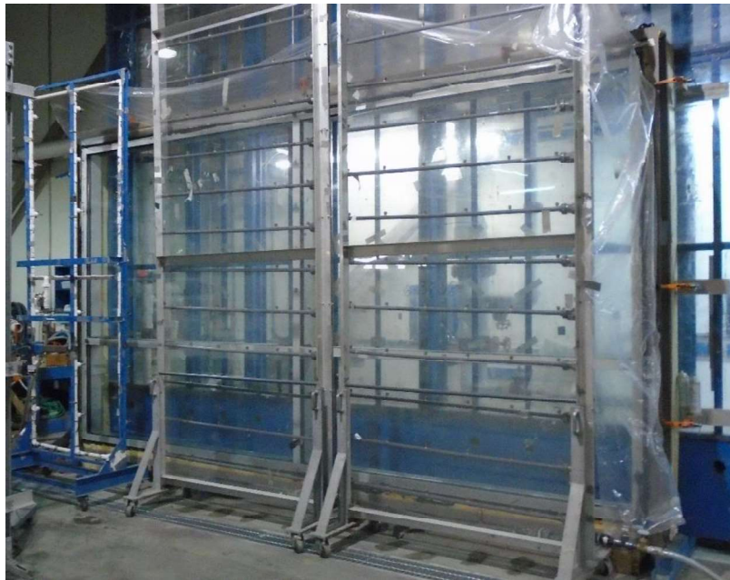
Photo No. 3 Test Specimen #1 during water penetration
