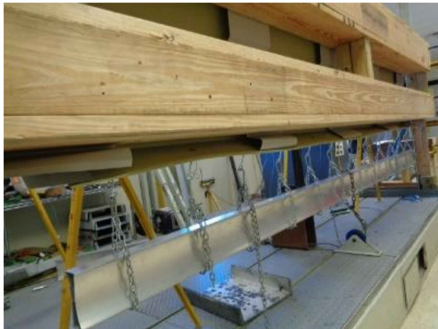
Photo No. 4 Typical Failure Mode - Coping System (32 in Wide Rapid-Lok Coping)
