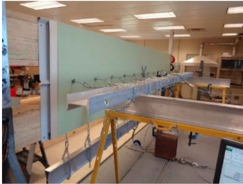
Photo No. 3 Typical Test Setup - Coping System
