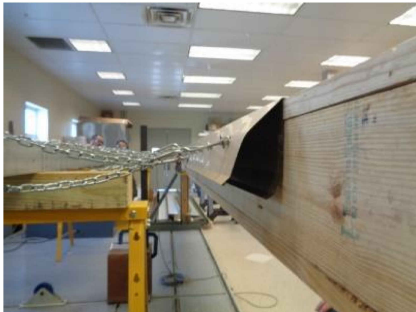
Photo No. 2 Typical Failure Mode - Fascia System
