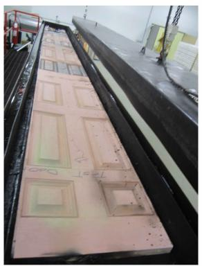
Photo No. 3 Unexposed Surface (Post Test)
