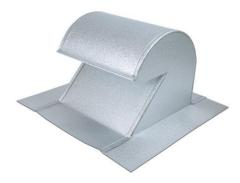
TAMCO Gooseneck Vent: Minimum 26 ga. ASTM A792 or ASTM A653 galvanized steel; F<sub>y</sub> = min. 50 ksi;
