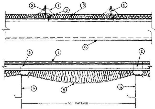
1. **Metal Roof Deck Panels\*** — For class 90—No. 24 MSG coated steel, for class 30—No. 26 MSG min. Coated steel. Panels continuous over two or more spans. End laps to occur adjacent to purlins with panels overlapped 3 inch max. A line of sealant may be used at panel end and side laps.
