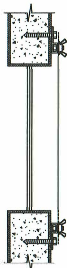
F-Track Typical Vertical Window Sectional View
