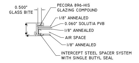
7/8" INSULATED ANNEALED IMPACT GLASS WITH 0.060" PVB INTERLAYER
