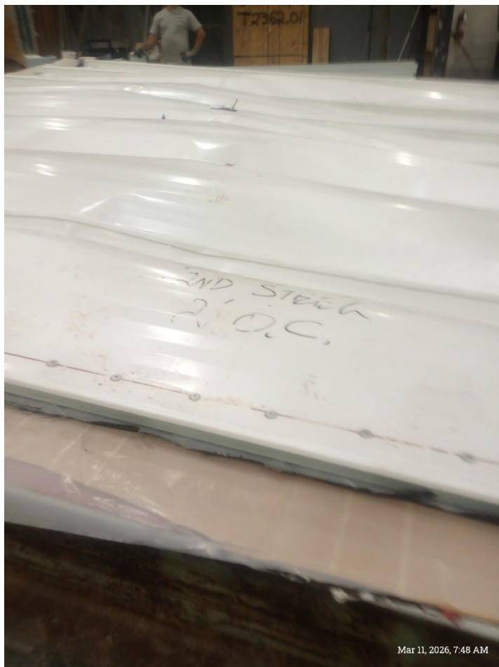
Photo No. 1 Steel Deck After Testing
