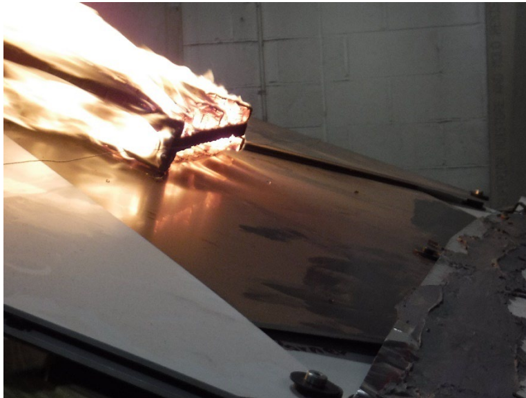
Photo No. 10 Test #2 Warping of Center ACM at Leading Edge
