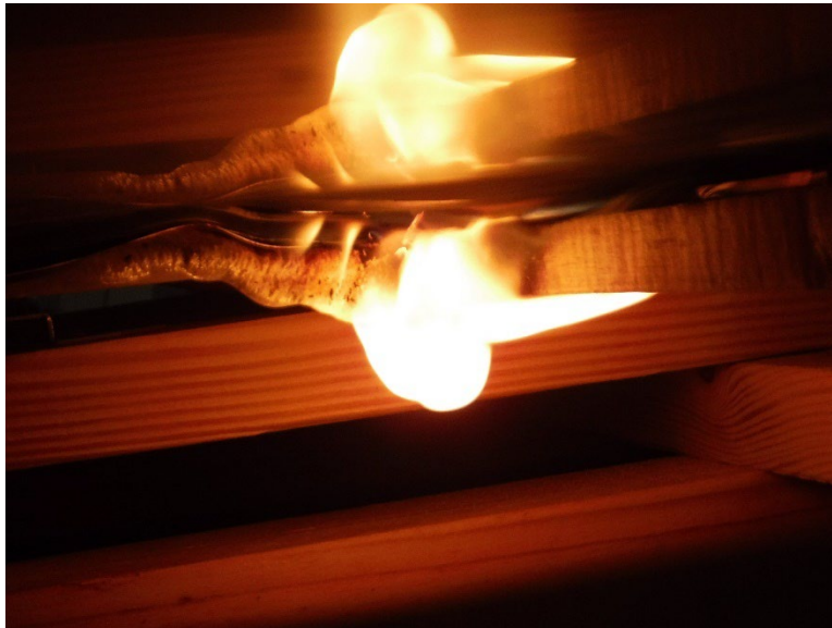
Photo No. 22 Test #4 Flaming of 1 x 4 Batten at Edge of ACM Underside of Panel
