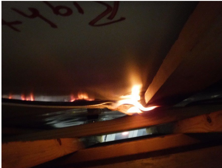
Photo No. 4 Test #1 Flaming of 1 x 4 Batten
