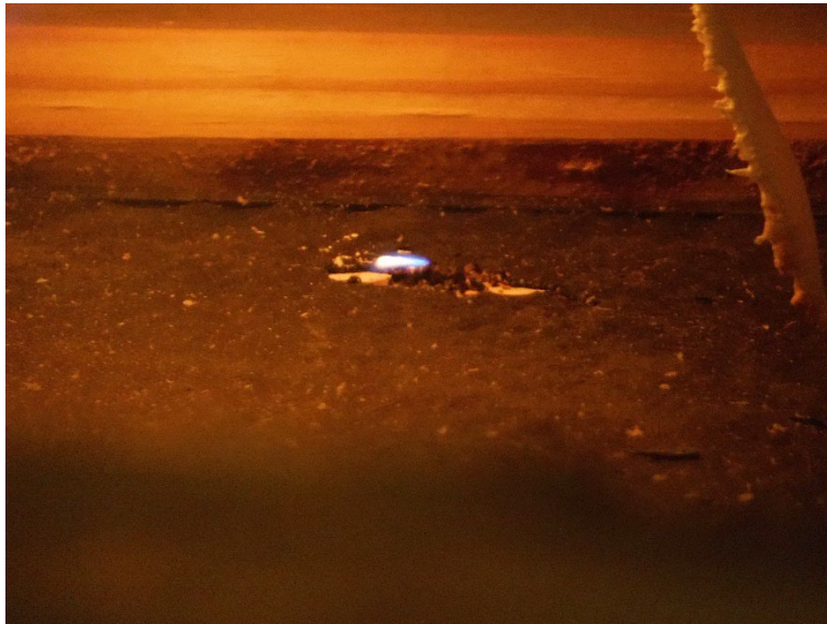
Photo No. 16 Test #3 Flaming Droplets from ACM onto Roof Deck
