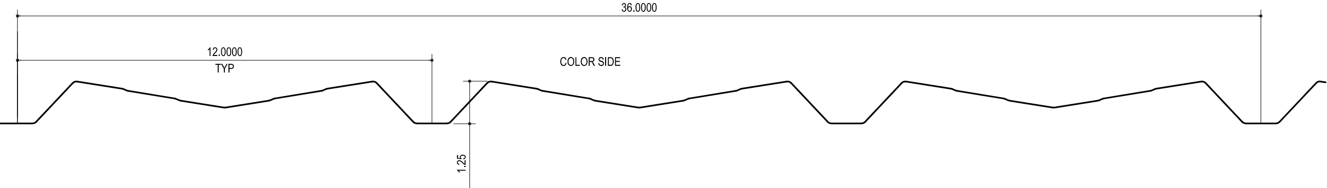
TYPICAL PANEL CROSS-SECTION 24 GA. ALUMINUM/ZINC COATED STEEL WITH PAINTED FINISH
