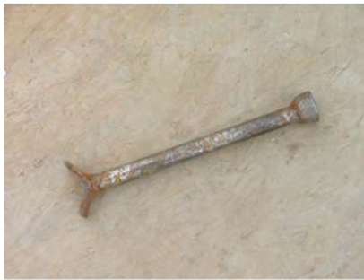
Leveling Angle Driver (Clavo para Ángulo de Nivel) - Used to set Leveling Angles to the required location without damage to the Leveling Angle.
