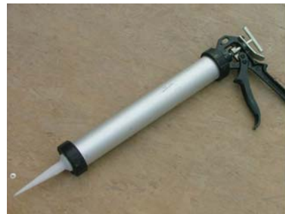
Sealant Sausage Gun 20 oz. (Aplicador de Pegamento) - (Sausage Style) Used to apply sealant.
