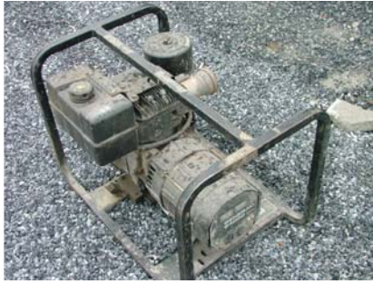
Generator (Generador) - Used as a source of electric for power tools and lights.
