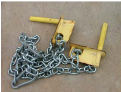
Safety Chains (Cadenas de Seguridad) - Used when offloading panels from trailer.
