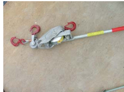
Come-Along (Cabrestante) - Used to draw panels together.
