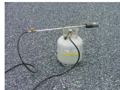
Torch - propane (Antorcha - propano)- Used to remove moisture from area of panel where sealant is to be applied.
