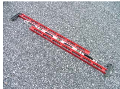
Level (Plumb-it Level) (Nivel) - Used to check panels for plumb.
