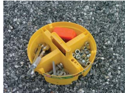
Tool Tray (Caja de Herramientas)- Used to carry tools, nuts, bolts, etc. on the jobsite.
