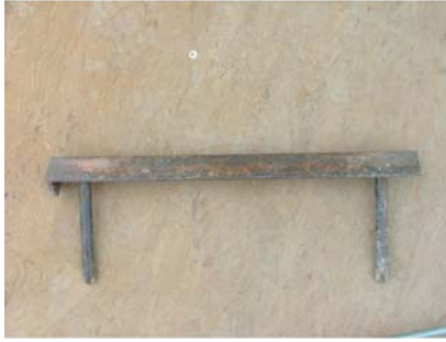
Leveling Angle (Ángulo de Nivel) “Screed Irons”- Set in the crushed stone at the required level, prior to screeding, to provide a screed guide.
