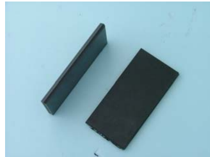
Plastic Shim Stock (Cuñas) - Must be min. 5,000 PSI plastic. Used as spacers to level a panel on a support ledge.
