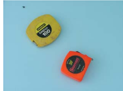
Tape Measure (Cinta Metro)- (30 ft. - 100 ft. - 300 ft.) Steel tapes are recommended. Tapes made of fabric or vinyl can stretch, causing inaccurate measurements.
