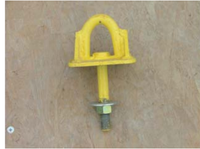
I-Bolt (Gancho) - Used to lift panels when SL Anchors are not available.
