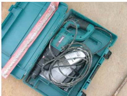
Hammer Drill (Taladro de Martillo) - Used for drilling through concrete.
