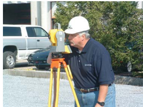
Figure 3.2 A Total Station can provide for a quick and accurate layout.
