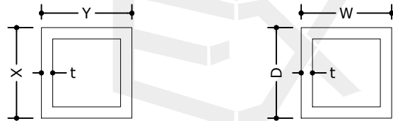
13 TRAP MOUNT TUBE, TYP. NOT TO SCALE 6063-T6 ALUM.
