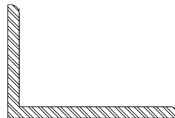
Part No. 30-0-276-X Item Description: 6063-T5 ALUMINUM CORNER PROFILE 120X80X8
