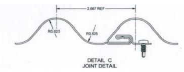
Typical Assembly Concealed Fastener Panel Interlock (Fasteners attached at 1-1/4" along the support span, in the concealed fastener panel interlock)
