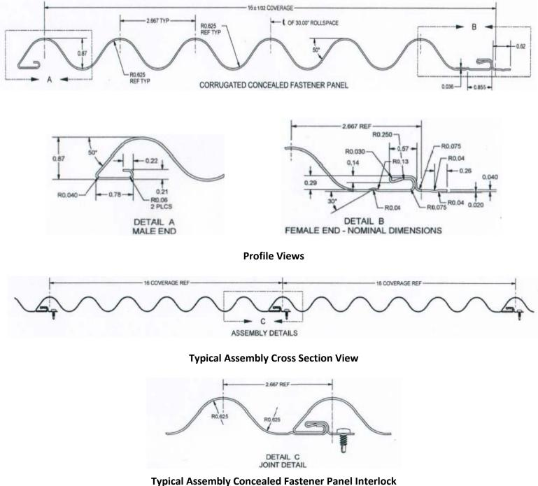
(Fasteners attached at 1-1/4" along the support span, in the concealed fastener panel interlock
