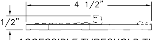
ACCESSIBLE THRESHOLD TH425 ALUMINUM 6063-T5
