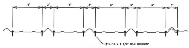
STANDARD FASTENER PATTERN @ 24" O.C. AND PANELS ENDS
