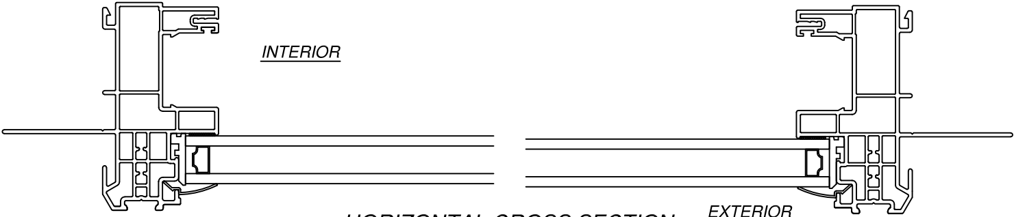
HORIZONTAL CROSS SECTION FIN INSTALLATION WITHOUT J-CHANNEL
