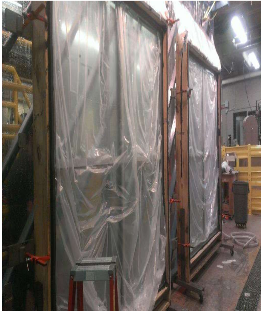
Photo No. 1 Unit During Air Infiltration
