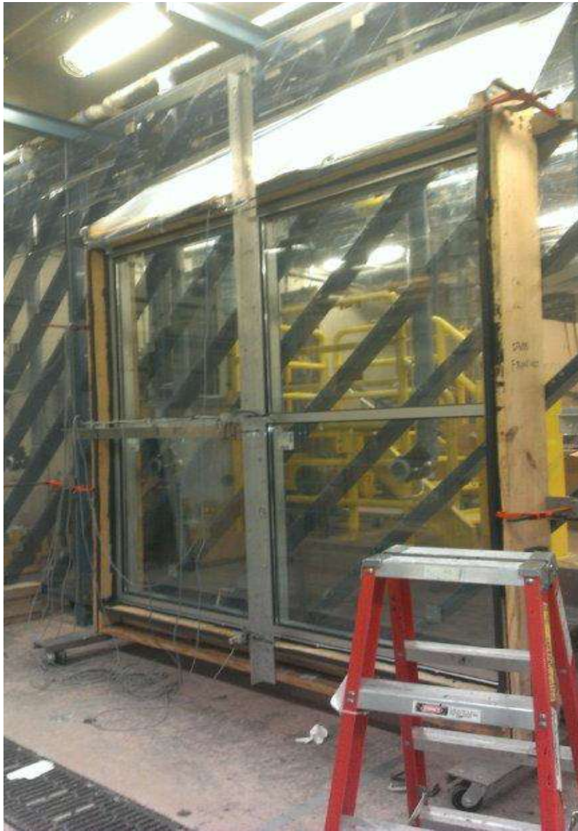
Photo No. 3 Unit During Uniform Static Load Infiltration
