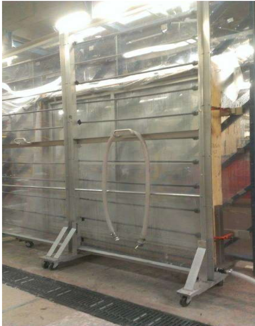
Photo No. 2 Unit During Water Infiltration
