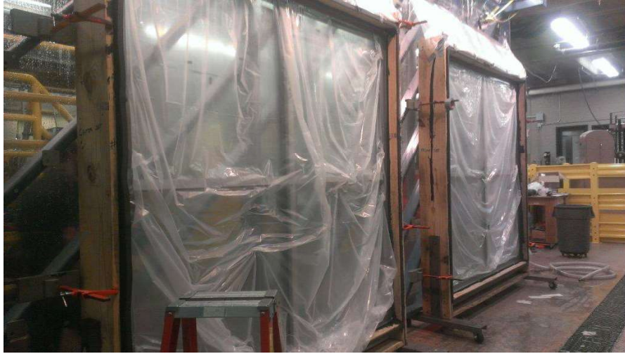
Photo No. 2 Unit During Air Infiltration
