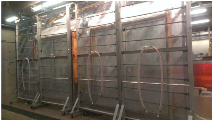
Photo No. 3 Unit During Water Infiltration
