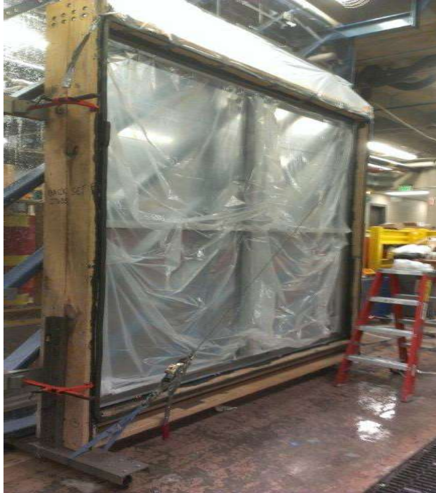
Photo No. 1 Unit During Air Infiltration
