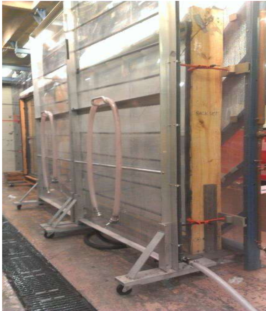
Photo No. 2 Unit During Water Infiltration
