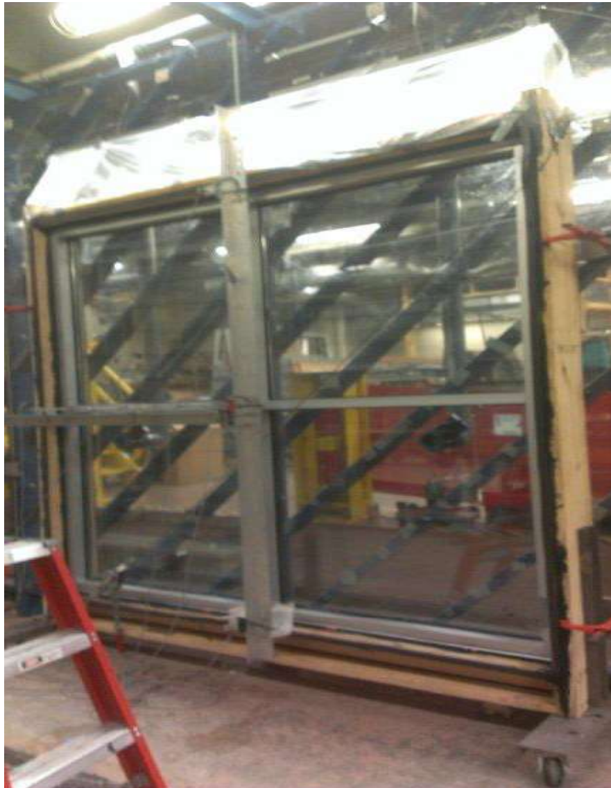
Photo No. 3 Unit During Uniform Static Load Infiltration
