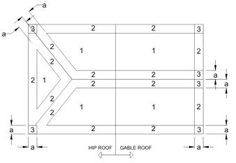
a: 10% OF LEAST HOIZONTAL DIMENSION OR 0.4h, WHICHEVER IS SMALLER, BUT NOT LESS THAN EITHER 4% OF LEAST HORIZONTAL DIMENSION OR 3FT (0.9M). OR AS DETERMINED BY DESIGN OR OTHER APPLICASALE CODE.
