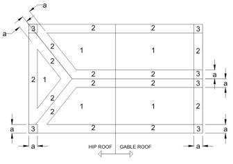
a: 10% OF LEAST HOIZONTAL DIMENSION OR 0.4h, WHICHEVER IS SMALLER, BUT NOT LESS THAN EITHER 4% OF LEAST HORIZONTAL DIMENSION OR 3 FT (0.9M). OR AS DETARMINED BY DESIGN OR OTHER APPLICABLE CODE.
