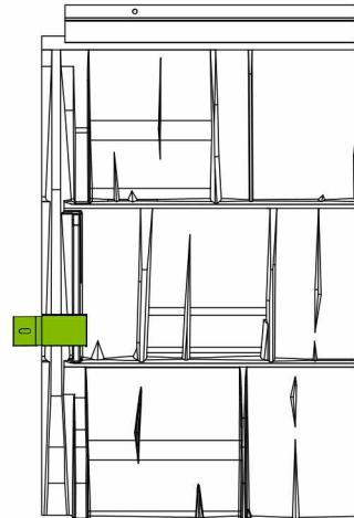
Clip placement on panel. The clip rests inside a recessed indent/pocket.
