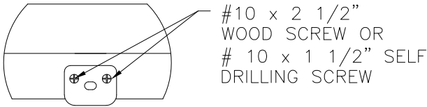
ASTRAGAL HEAD STRIKE DETAIL 2X BUCK/WOOD FRAMING OR METAL STRUCTURE
