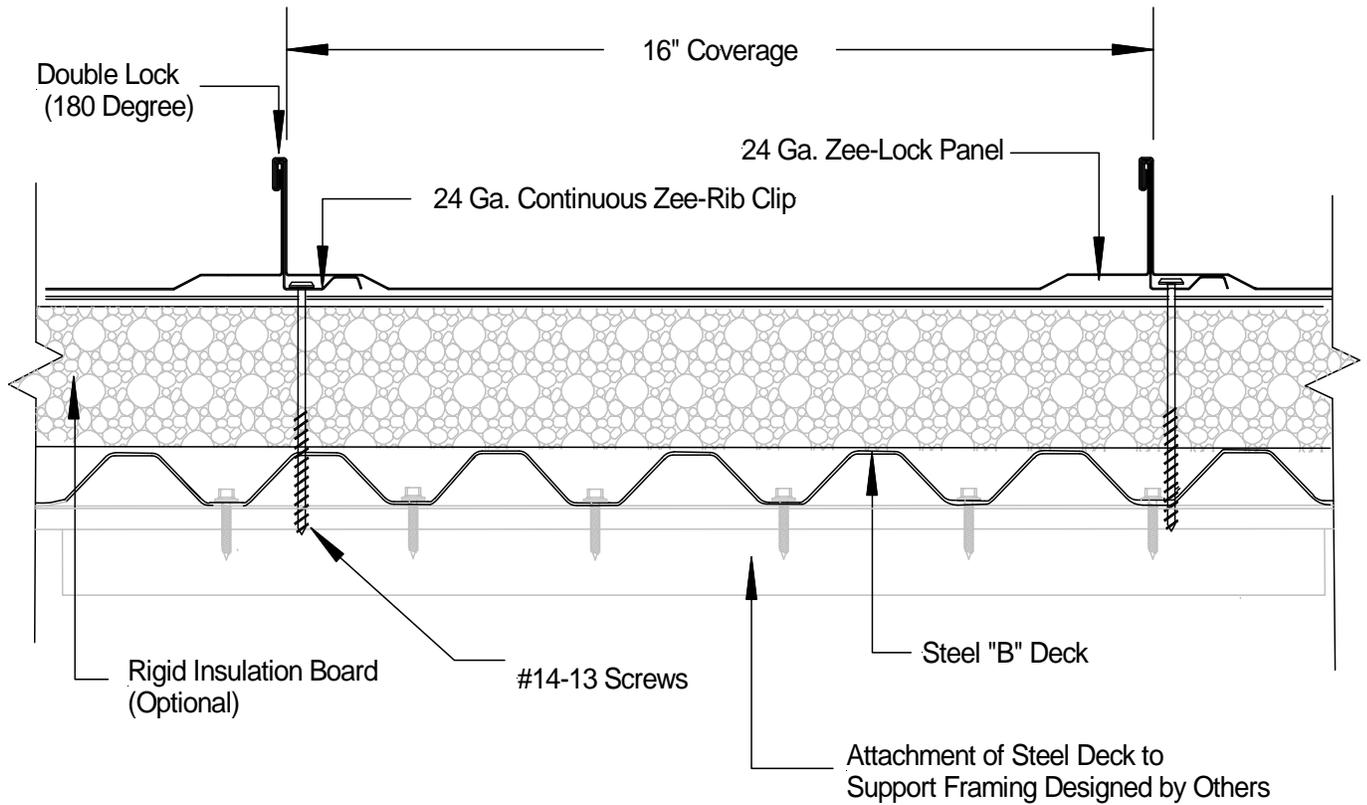
**"Zee-Lock" Panel attached to Steel Deck
