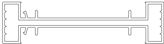
5000 FIN & J FRAME VINYL H-MULLION COVER #VPI-573 EXTRUDED VINYL 0.071" MIN.
