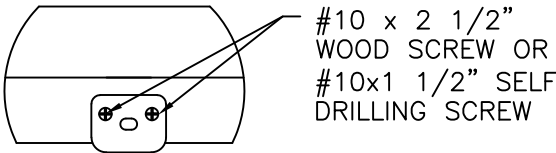
ASTRAGAL HEAD STRIKE DETAIL 2X BUCK/WOOD FRAMING OR METAL STRUCTURE
