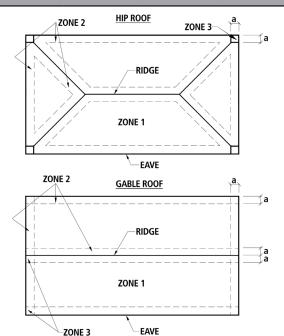
Note: Dimension (a) is defined as 10% of the minimum width of the building or 40% of the mean height of the roof, whichever is smaller, however, (a) cannot be less than either 4% of the minimum width of the building or 3 feet.
