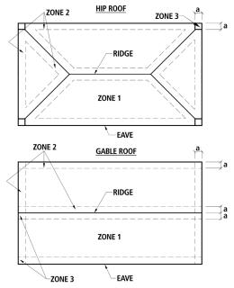
Note: Dimension (a) is defined as 10% of the minimum width of the building or 40% of the mean height of the roof, whichever is smaller, however, (a) cannot be less than either 4% of the minimum width of the building or 3 feet.
