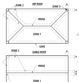
Note: Dimension (a) is defined as 10% of the minimum width of the building or 40% of the mean height of the roof, whichever is smaller, however, (a) cannot be less than either 4% of the minimum width of the building or 3 feet.
