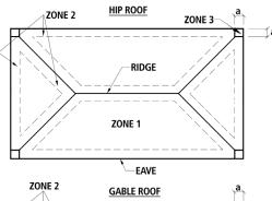
Note: Dimension (a) is defined as 10% of the minimum width of the building or 40% of the mean height of the roof, whichever is smaller, however, (a) cannot be less than either 4% of the minimum width of the building or 3 feet.
