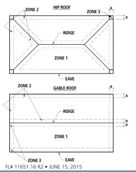
Note: Dimension (a) is defined as 10% of the minimum width of the building or 40% of the mean height of the roof, whichever is smaller, however, (a) cannot be less than either 4% of the minimum width of the building or 3 feet.
