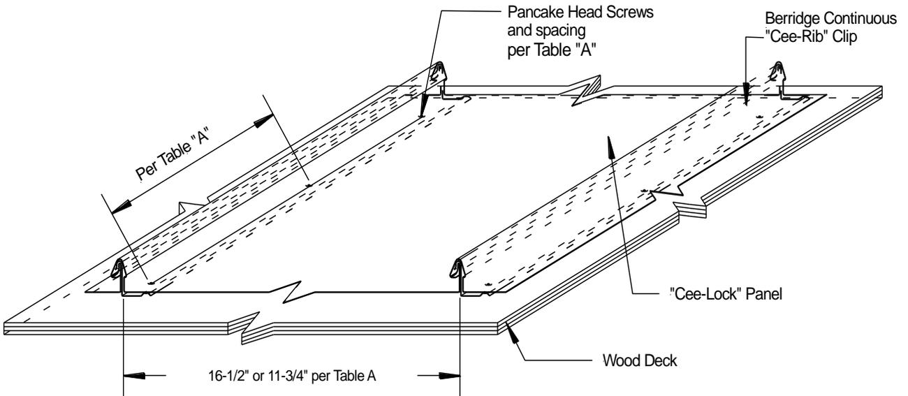
**Typical Roof Assembly with Berridge Continuous "Cee-Rib" Panel Clip - Isometric View**
