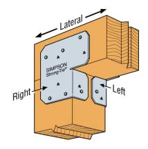
FIGURE 3a—AC POST CAP CONNECTOR COMPONENTS
