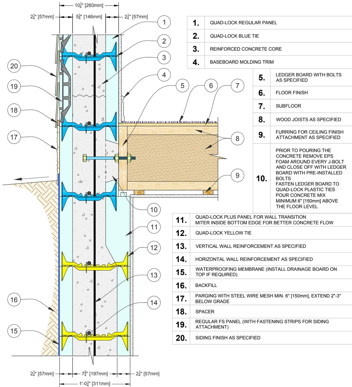
Figure 72: Wall Width Transition & Ledger Connection
