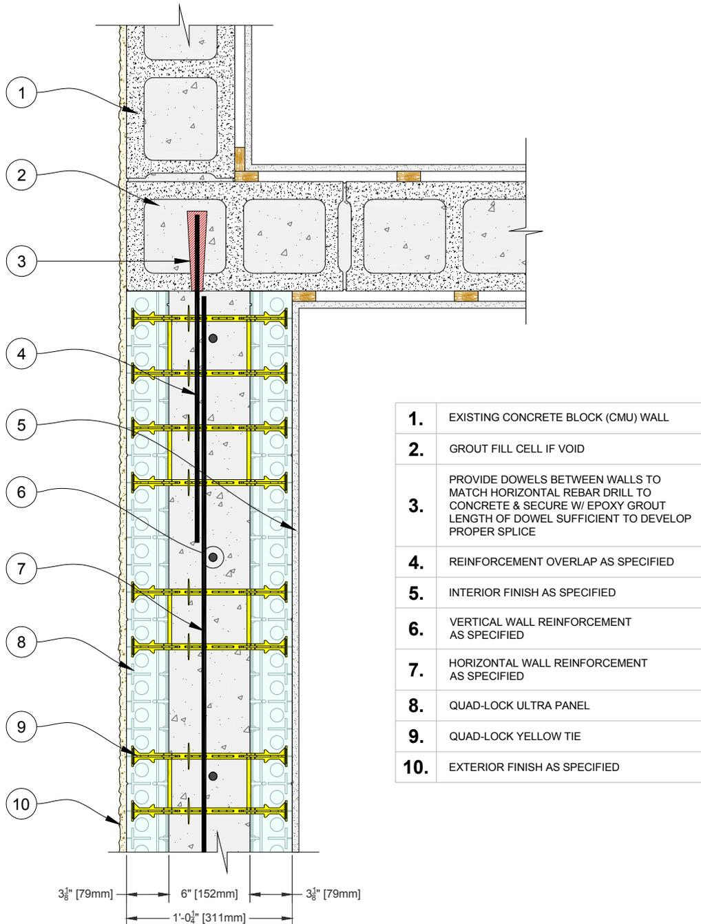
Figure 125: Typical Connection to Existing Concrete Wall (Plan View)
