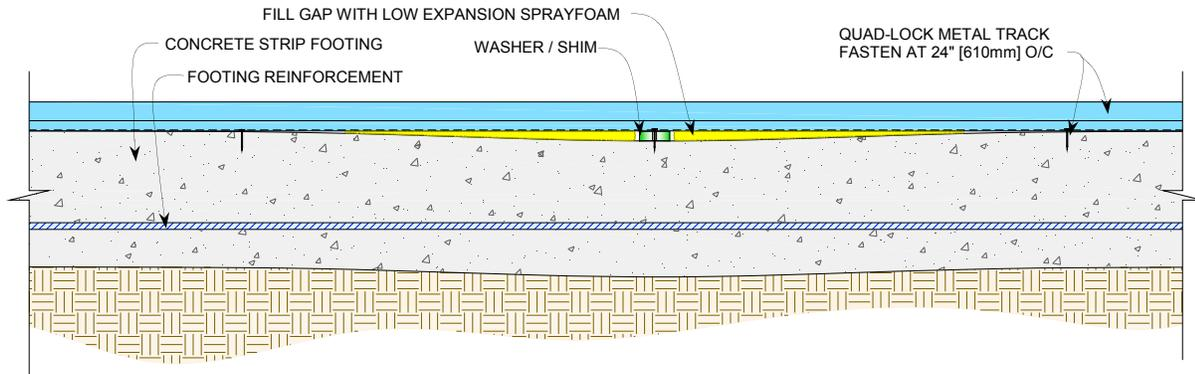
Figure 33: Dealing with Small Variations in Footing Elevations
