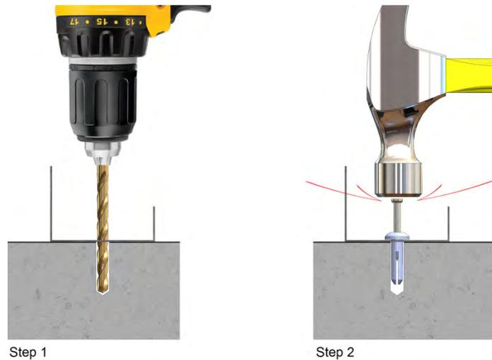
*Figure 39: Installation of Hit-Anchors*
