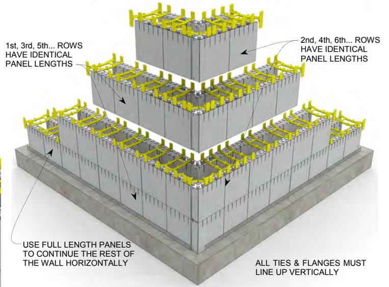
**STEP 8** R-28 [U-0.21] 6" [152mm] Concrete Wall (Alternate Method)
