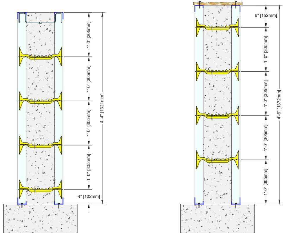
Figure 50: Panels Ripped to Adjust Wall Elevation
