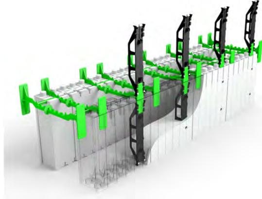
Figure 7: Quad-Lock 4" FS Panel
