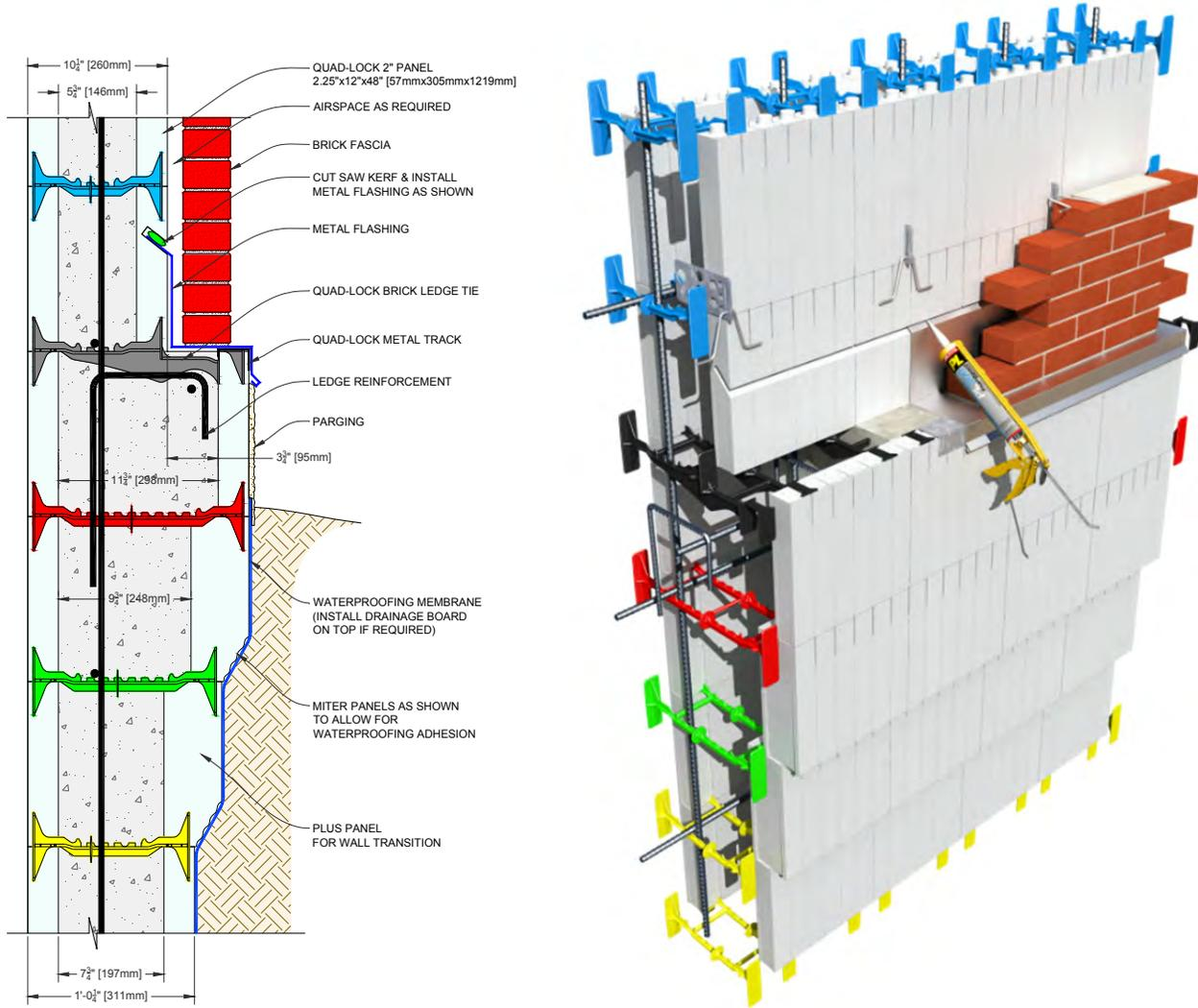
Figure 148: Brick Ledge with Quad-Lock Brick Ledge Tie
