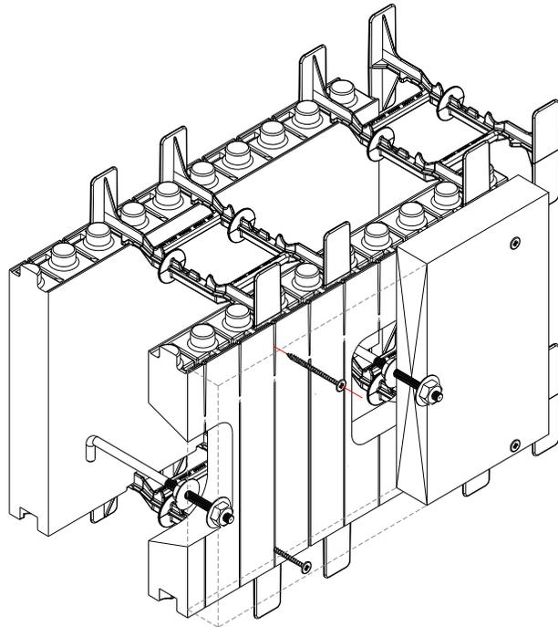
Figure 114: Typical Ledger Board Connection w/ Anchor Bolts
