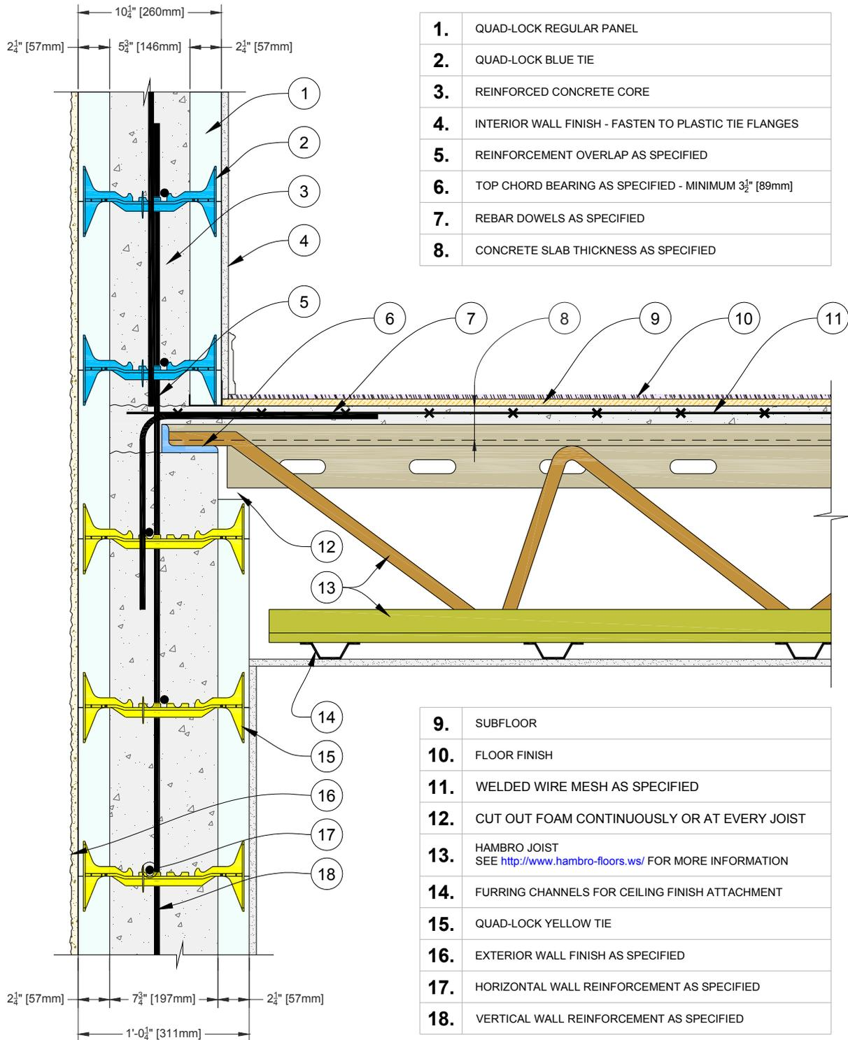
Figure 119: Typical Hambro Composite Floor System Connection
