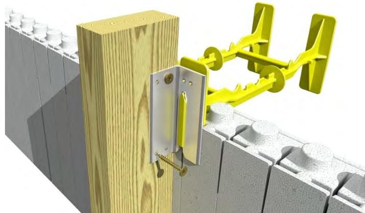
Figure 15: Slab Tie & Slab Bracket Assembly
