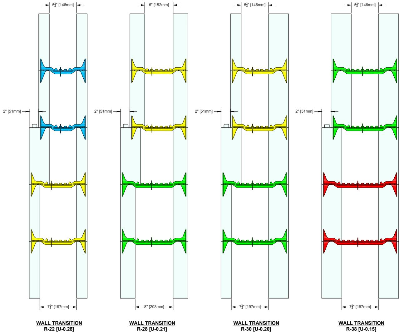
Figure 73: Wall Width Transition using Quad-Lock Plus Panels
