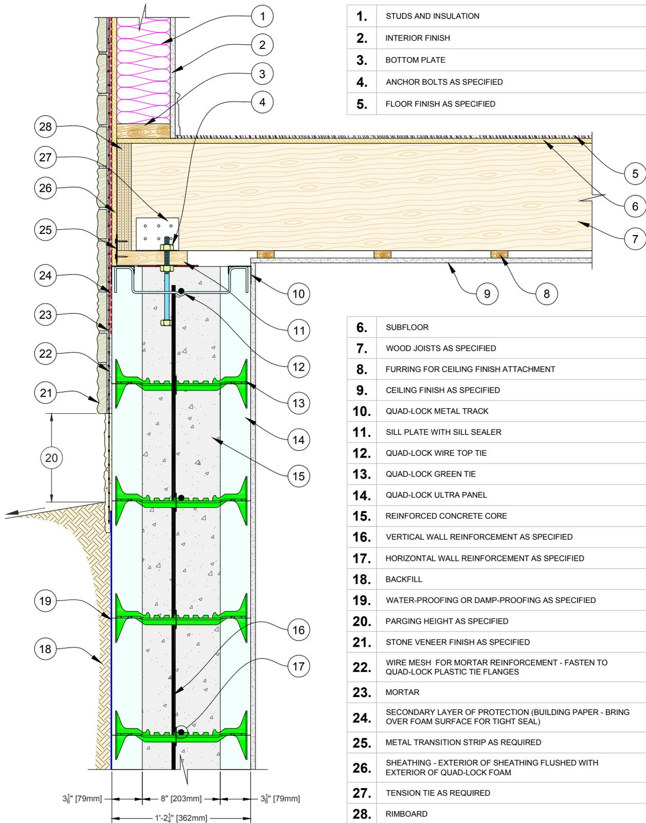
Figure 121: Typical Wall to Floor & Framing Connection
