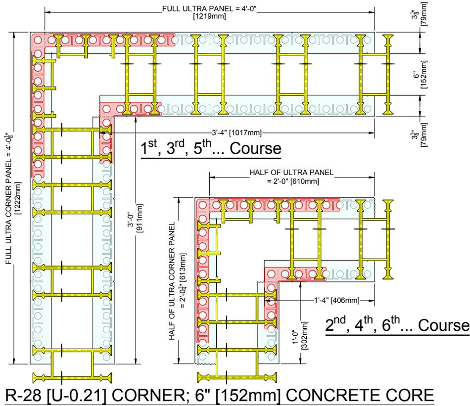
Figure 48: Panel/Tie Combination for R-28 [U-0,21] 6" Concrete Cavity
