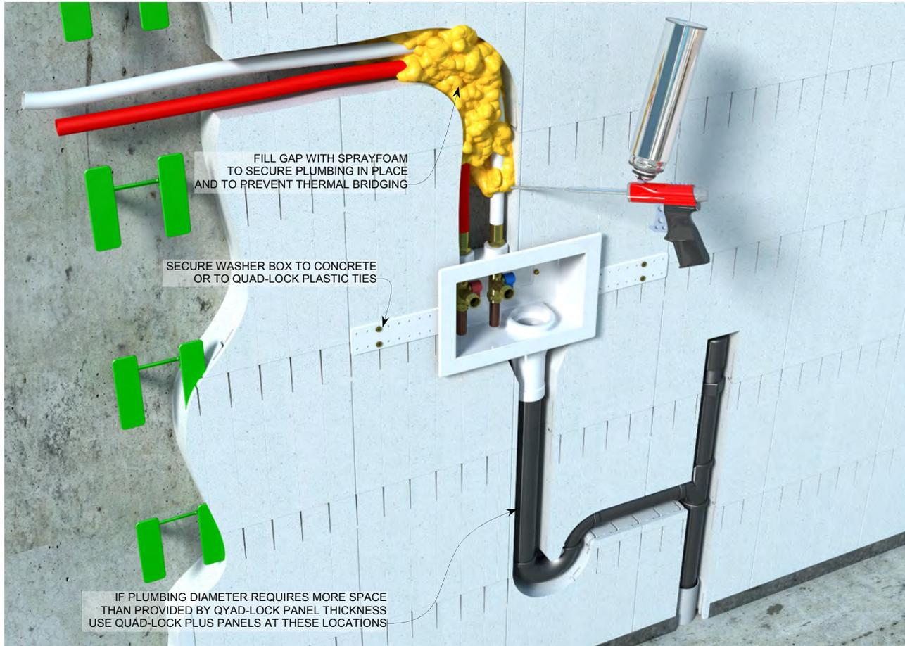
Figure 161: Plumbing Installation (After-Pour Method)
