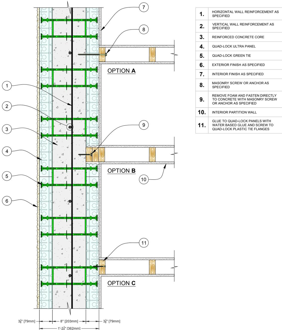
Figure 124: Typical Interior Partition Wall Connections (plan view)
