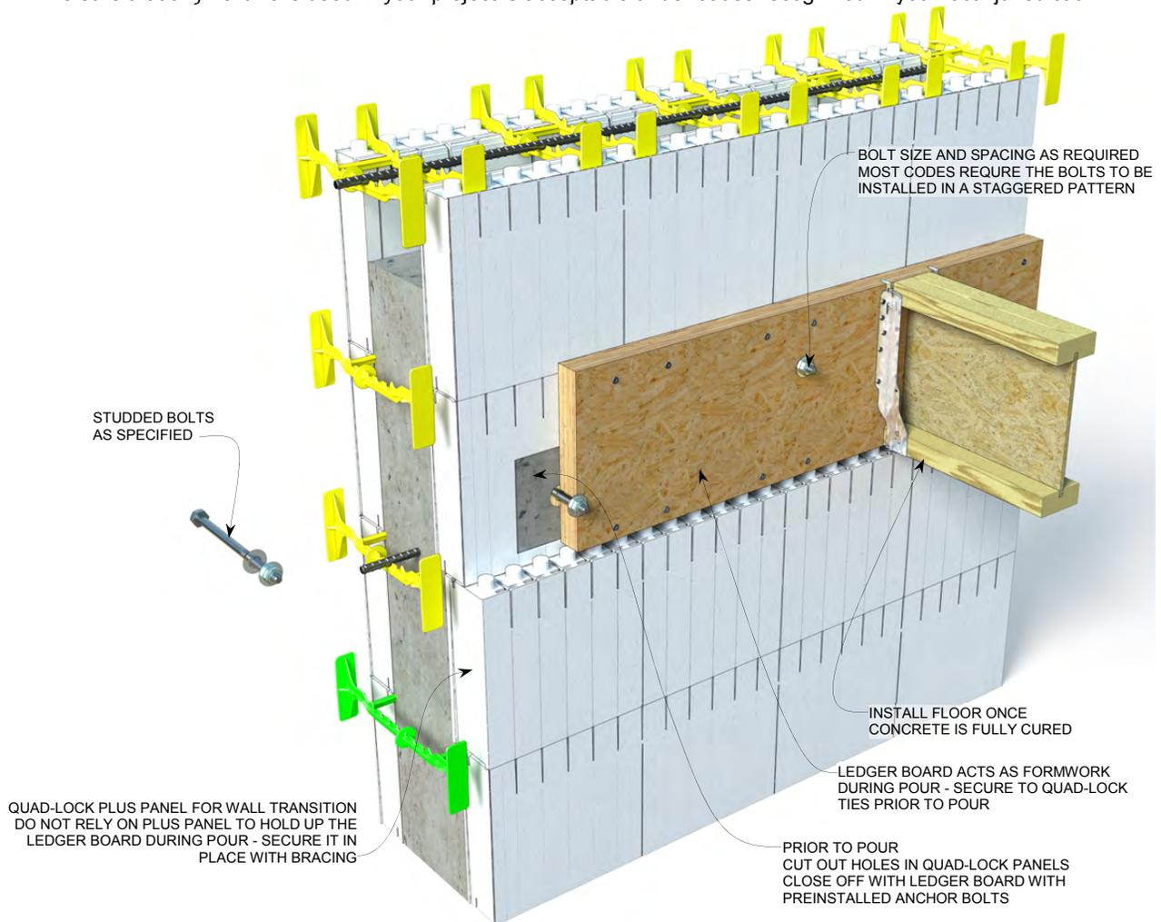
Figure 111: Installation of Floor Ledger Board
