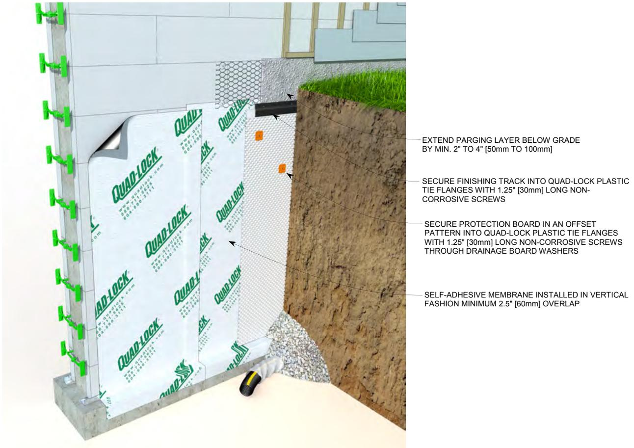
Figure 135: Water Proofing with Protection Board
