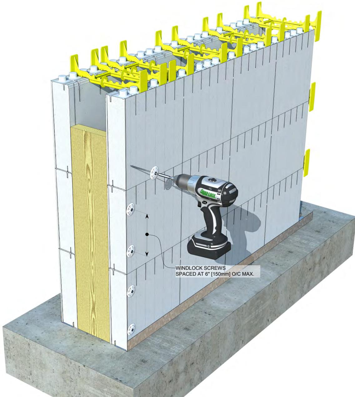
Figure 57: Bulkhead Formed with Lumber and Windlocks
