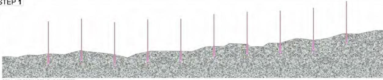
DRILL AND EPOXY REBAR AS SPECIFIED.
