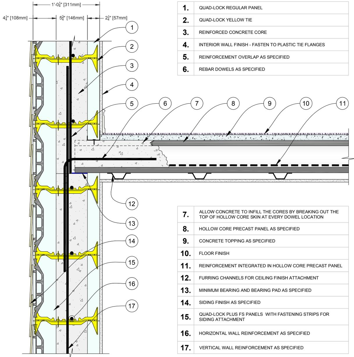
Figure 117: Typical Hollow Core Precast Floor Slab Connection
