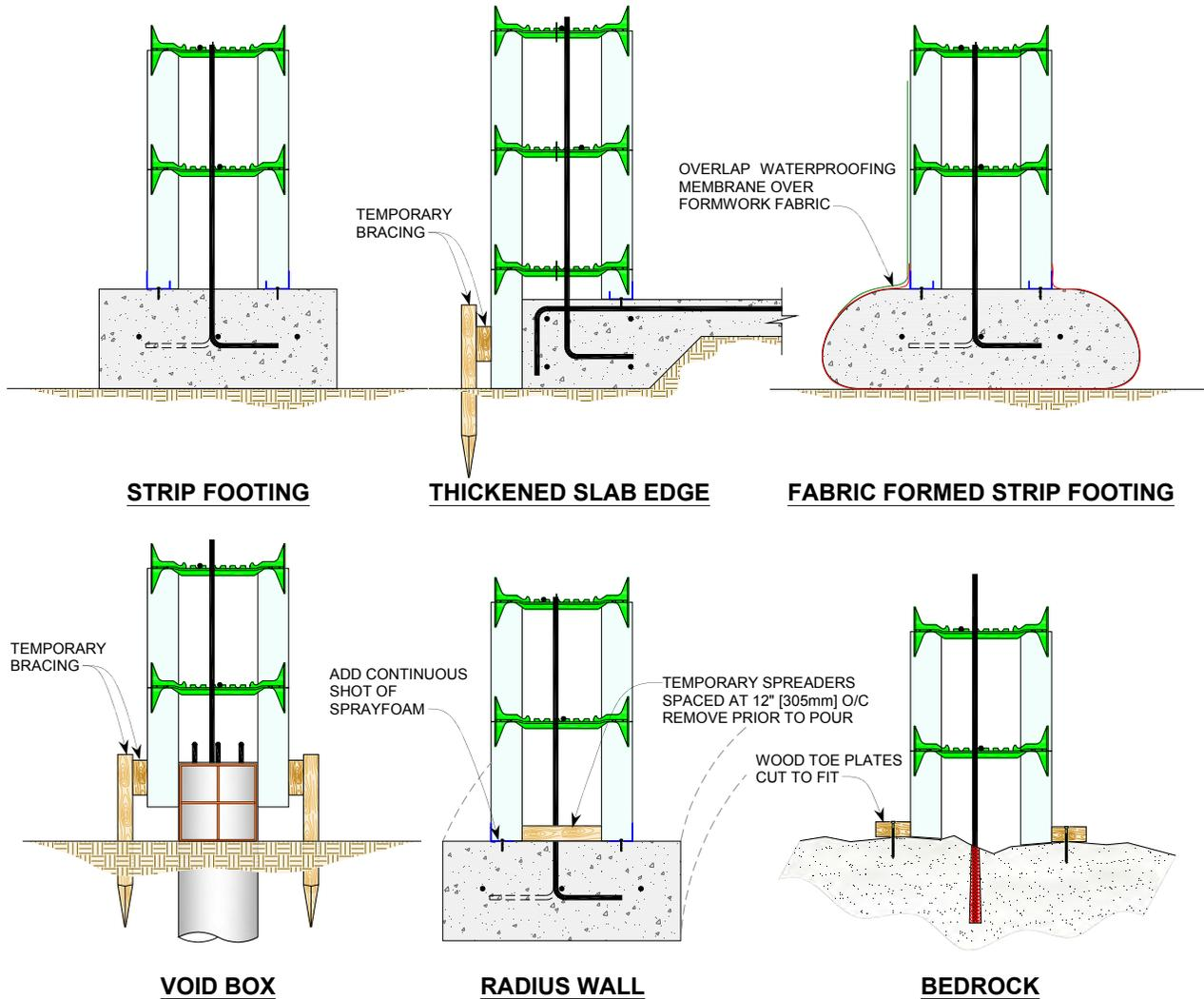
Figure 37: Typical Bottom of Wall Details
