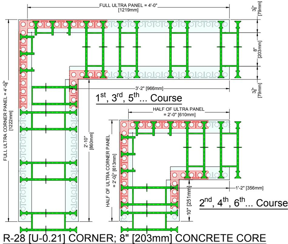
Figure 49: Panel/Tie Combination for R-28 [U-0,21] 8" Concrete Cavity
