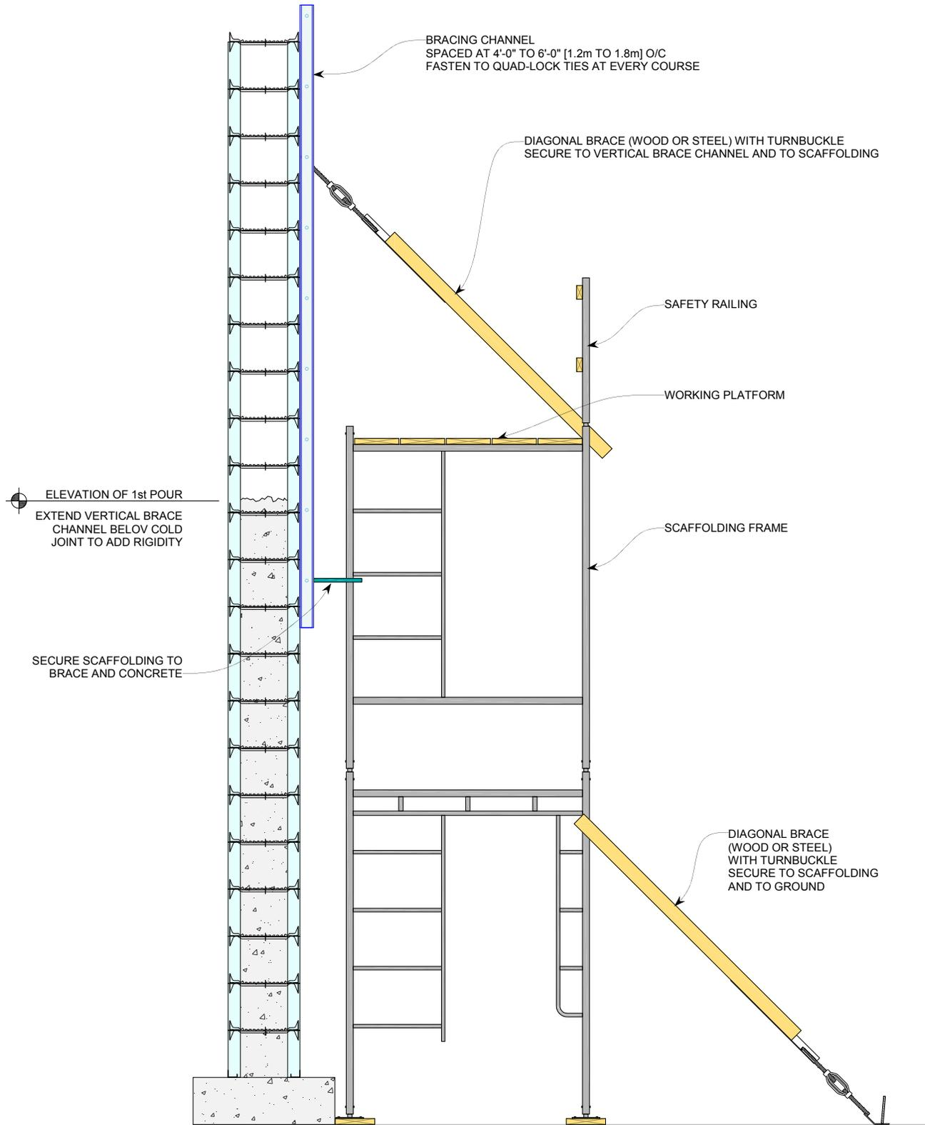
Figure 110: Bracing Tall Walls with Scaffolding
