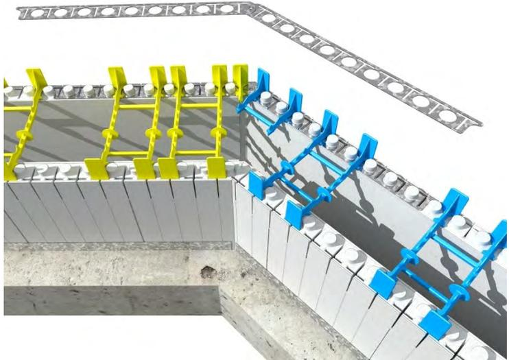
Figure 20: Assembly of Angle
