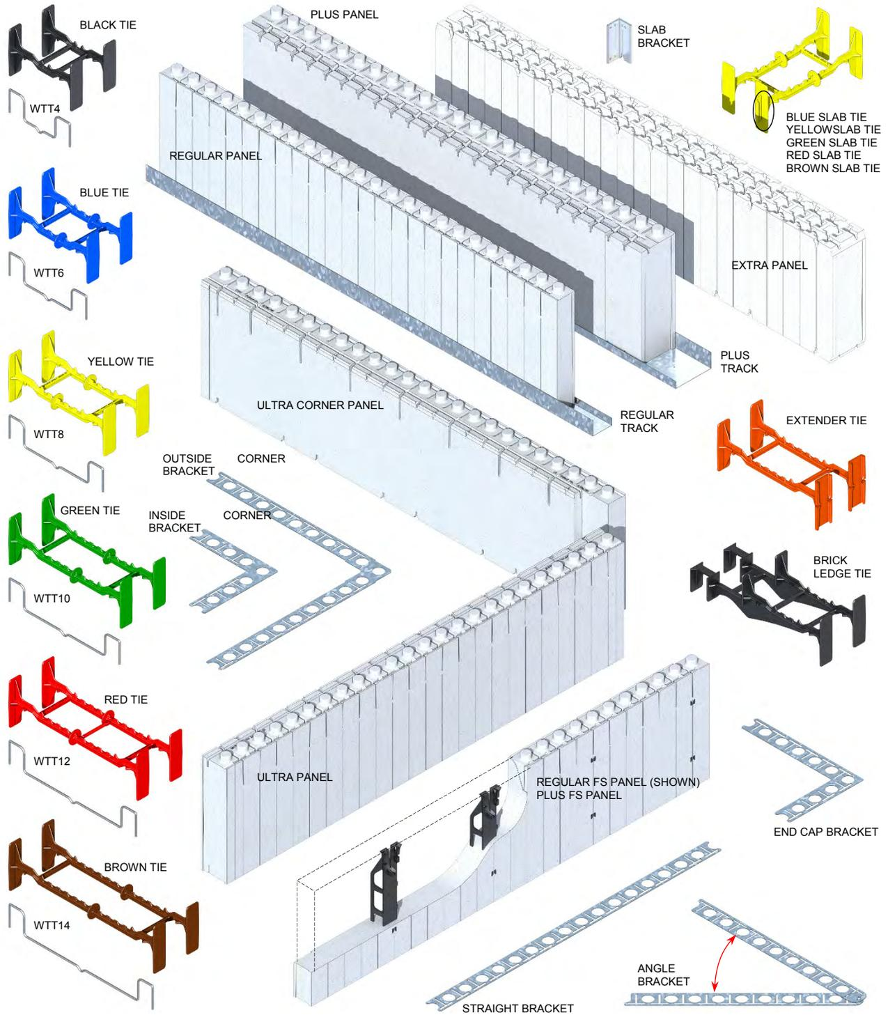
Figure 1: Quad-Lock Components
