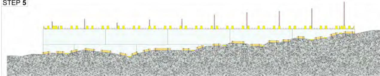
NAIL WOOD PLATES TO BEDROCK (TO BOTH SIDES OF WALL) TO SECURE QUAD-LOCK INTO PLACE. USE SPRAYFOAM TO SEAL OFF THE GAPS.
