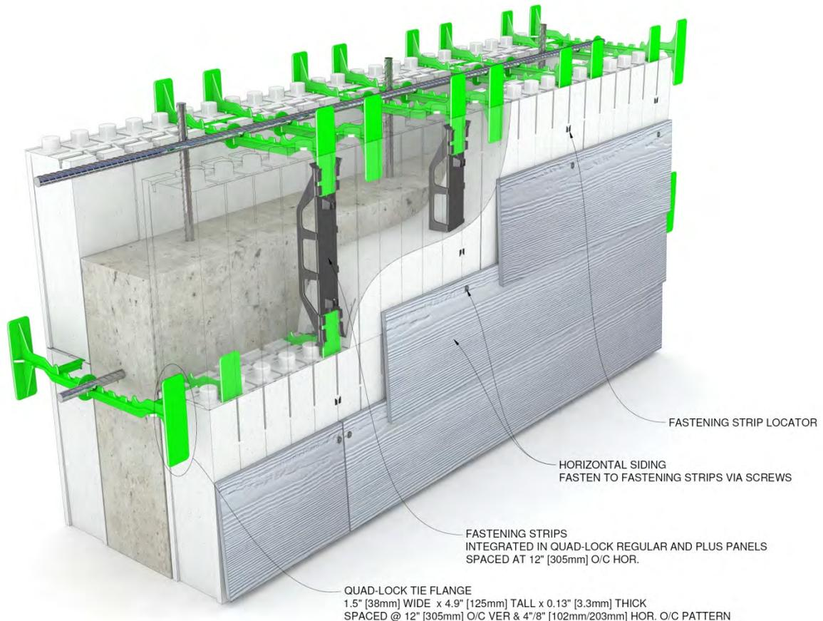
Figure 139: Cladding Details
