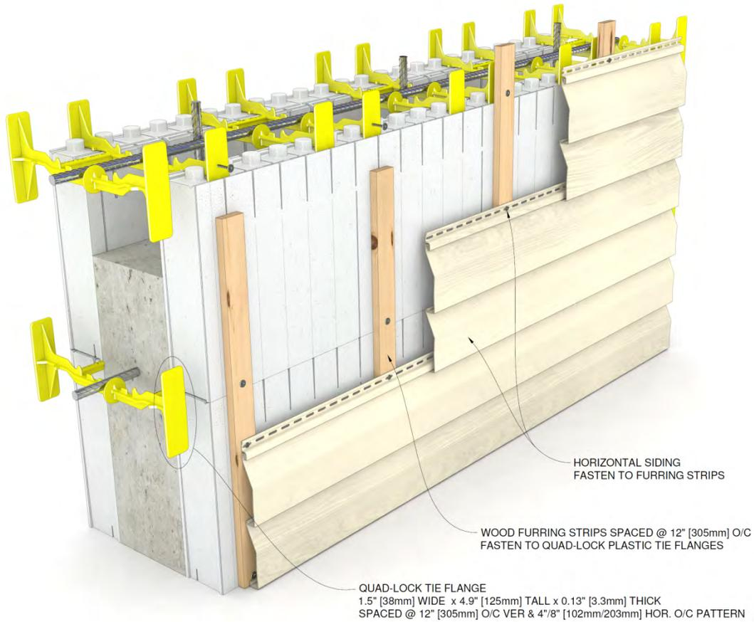
Figure 141: Siding Attachment with external furring strips
