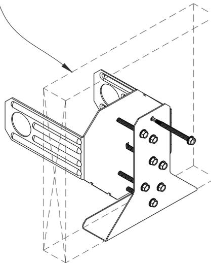
Figure 113: Ledger Installation using ICF Ledger Connectors
