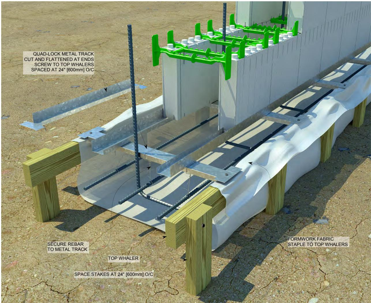
Figure 79: Typical Monolithic Footing / Wall Set Up
