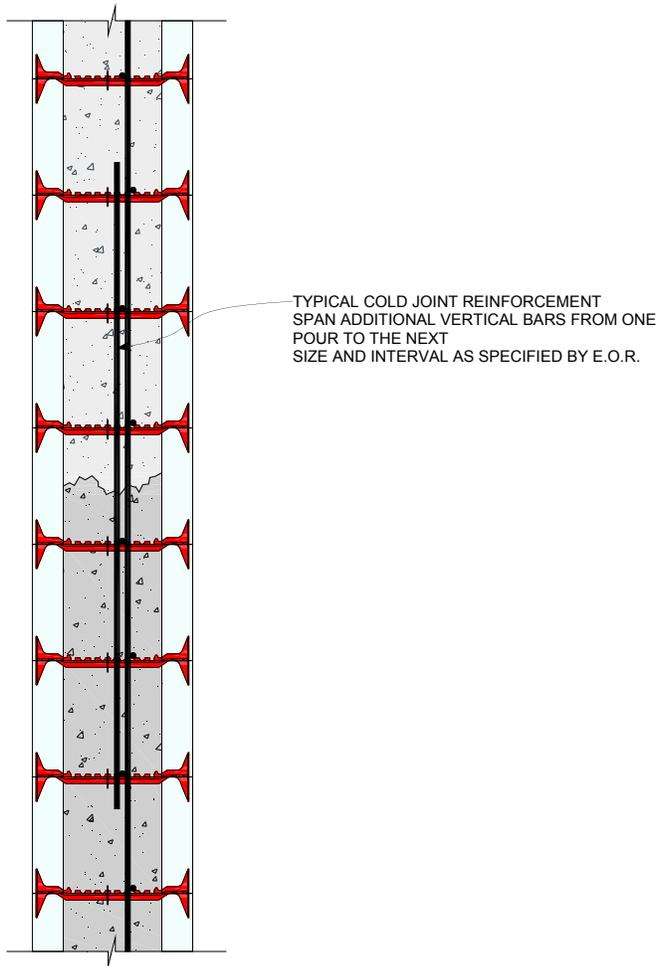
Figure 70: Cold Joint Reinforcement
