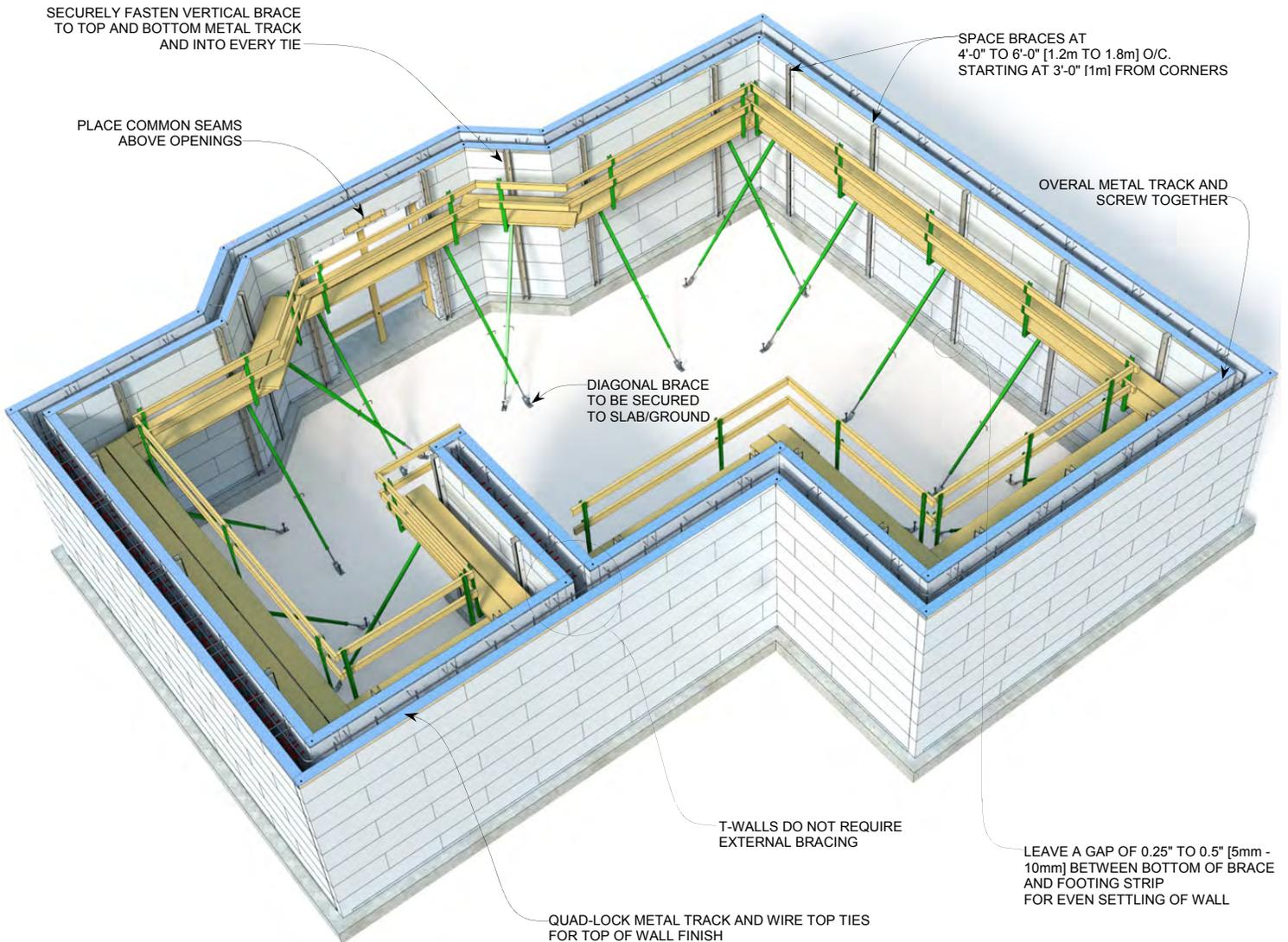
Figure 106: Metal Bracing System
