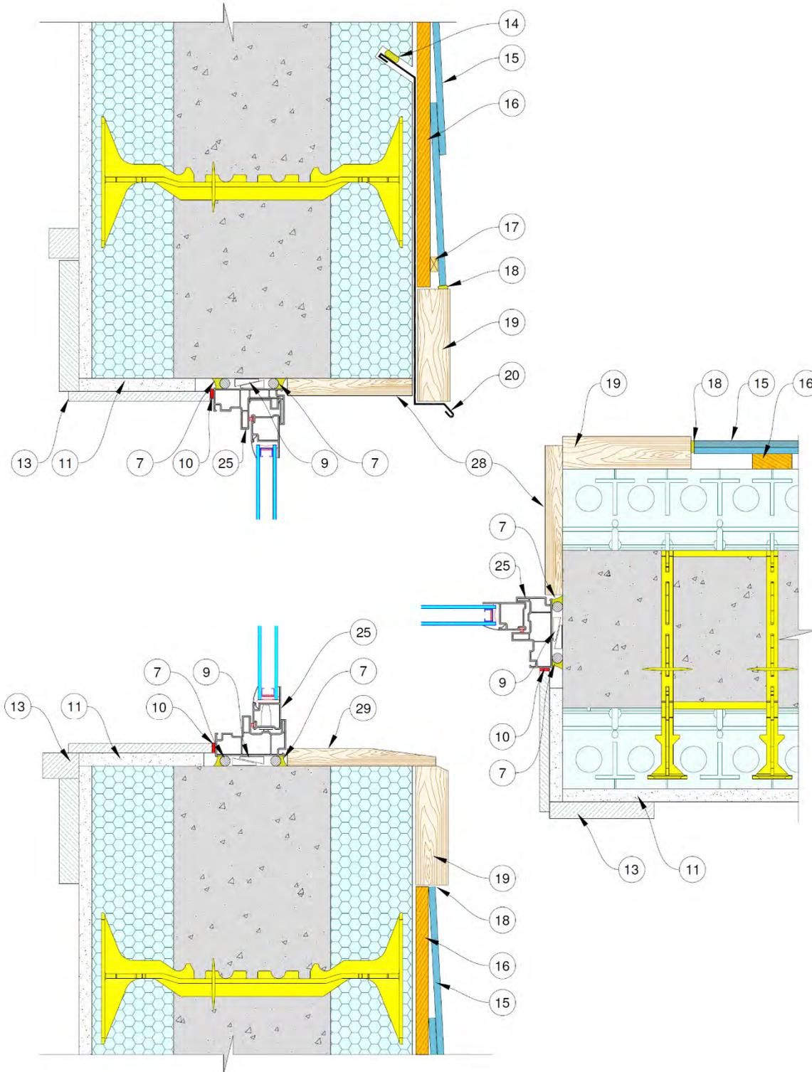
Figure 96: ICF Window Assembly - Direct to concrete, Boxed window centered, Lapped siding
