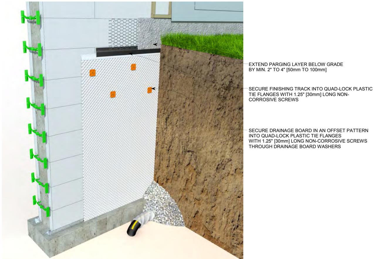
Figure 134: Damp Proofing with Drainage/Dimple Board
