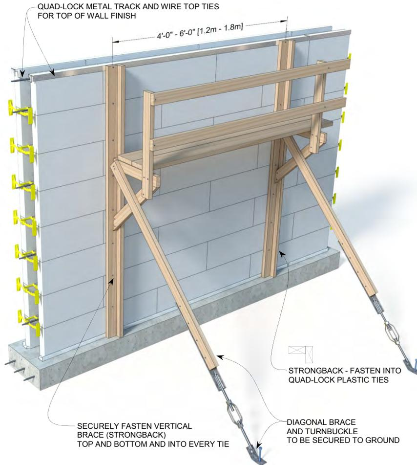
Figure 107: Site Constructed Wood Wall Bracing
