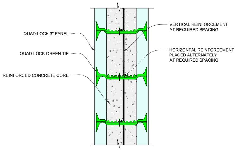
Figure 131: Rebar Placement
