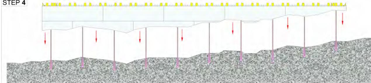
CUT OFF THE PART BELOW THE SCRIBED LINE, REMOVE WOOD PLATFORM AND FIT QUAD-LOCK ONTO BEDROCK
