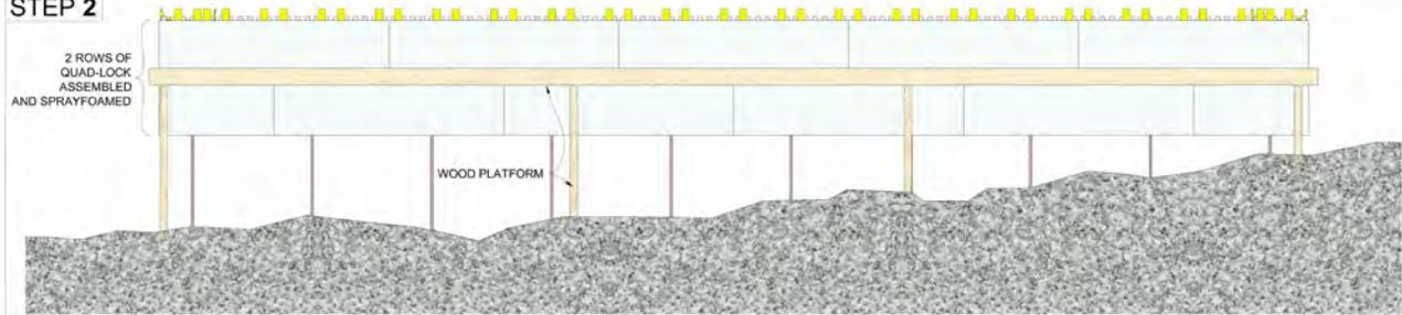
CONSTRUCT TEMPORARY LEVELED WOOD PLATFORM AND ASSEMBLE 2 ROWS OF QUAD-LOCK AS SHOW. SPRAYFOAM QUAD-LOCK PANELS TOGETHER INTO ONE SOLID PIECE
