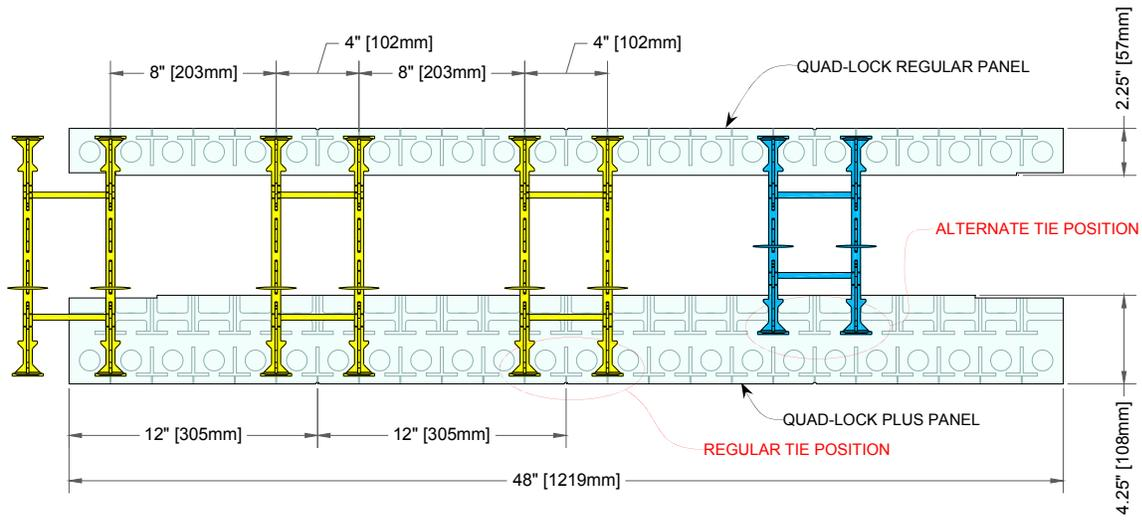
Figure 11: Quad-Lock Plus Panel - Positioning of Ties
