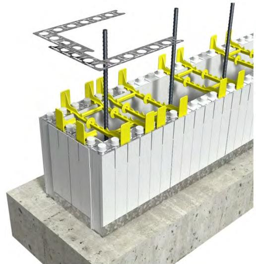
Figure 22: End Cap (Bulkhead) Assembly with End Cap Brackets
