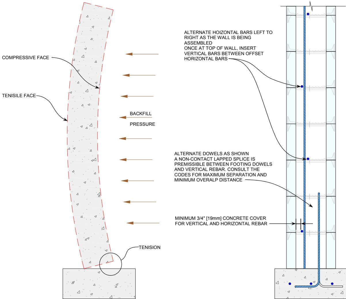
Figure 127: Position of Reinforcement within Quad-Lock Walls
