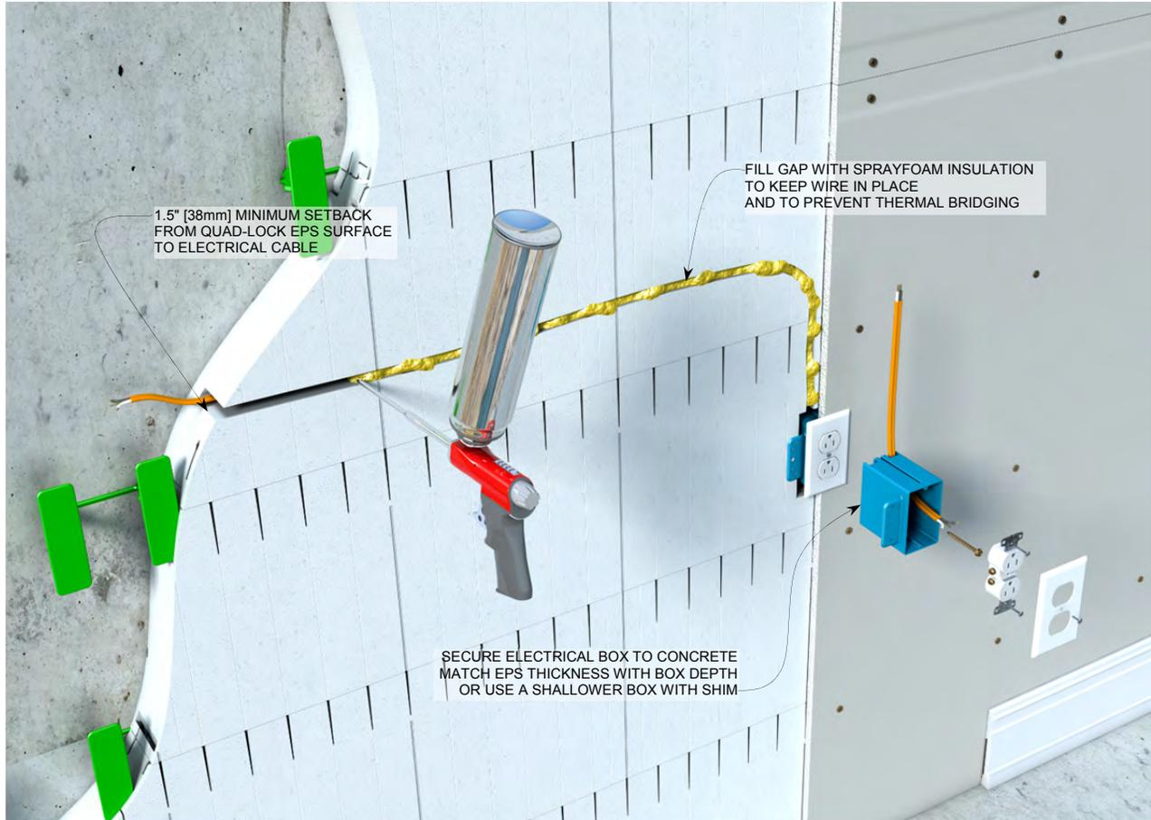
Figure 160: Installation of Electrical Boxes and Wiring
