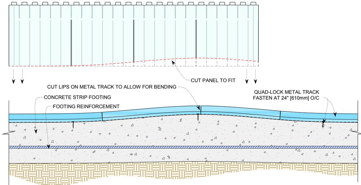
Figure 34: Adapting panels to inconsistencies in footing elevation
