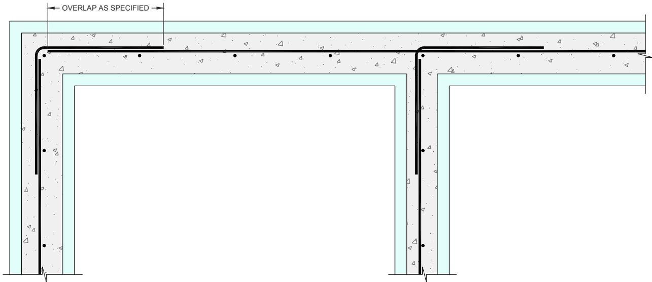
Figure 130: Typical Lap Patterns at Corners & T-Walls
