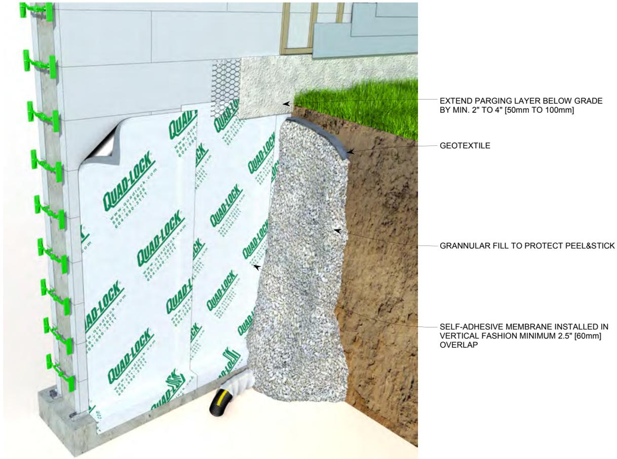
Figure 136: Water Proofing with Peel&Stick
