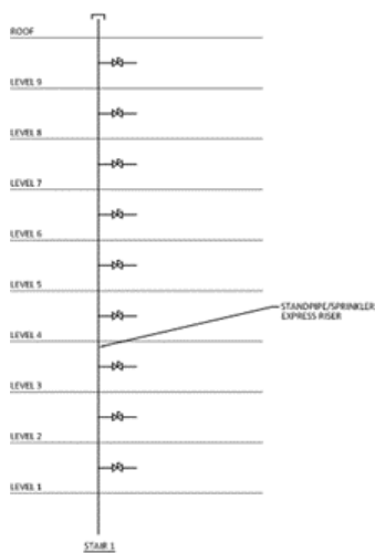
Figure 1. Sprinkler express risers or standpipes in high-rise buildings having a building height less than 420 ft.
