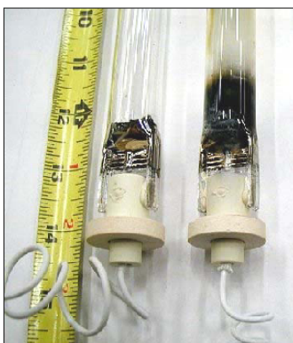
Figure 2.17. Aged UV Lamp (right) Compared to a New UV Lamp (left)
