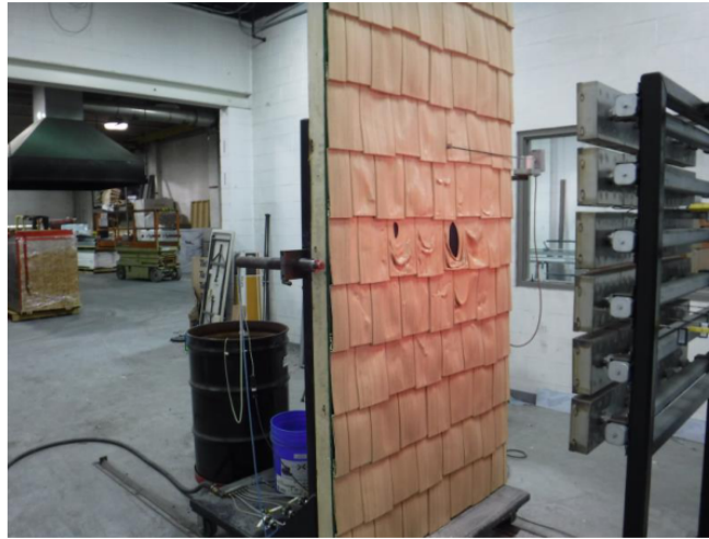
Photo No. 5 Melting of Exposed Surface
