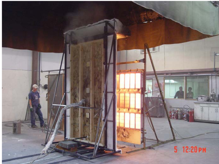
FIGURE 3. START OF TEST. WATER COOLED SHIELD IN FRONT OF ICAL HAS BEEN PULLED AWAY.
