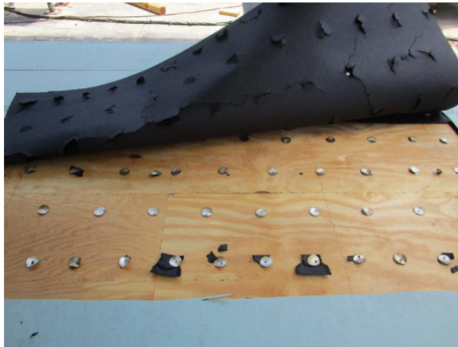
Specimen #2 failure – fastener pull-through
