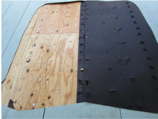
Specimen #1 failure – fastener pull-through
