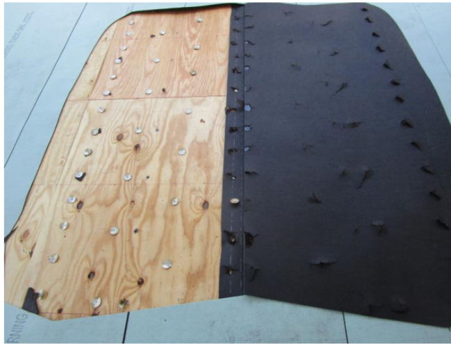
Specimen #1 failure – fastener pull-through
