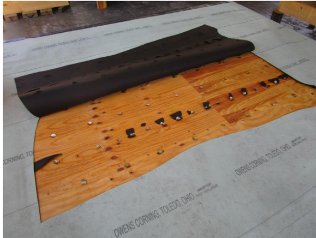
Specimen #4 failure – fastener pull-through
