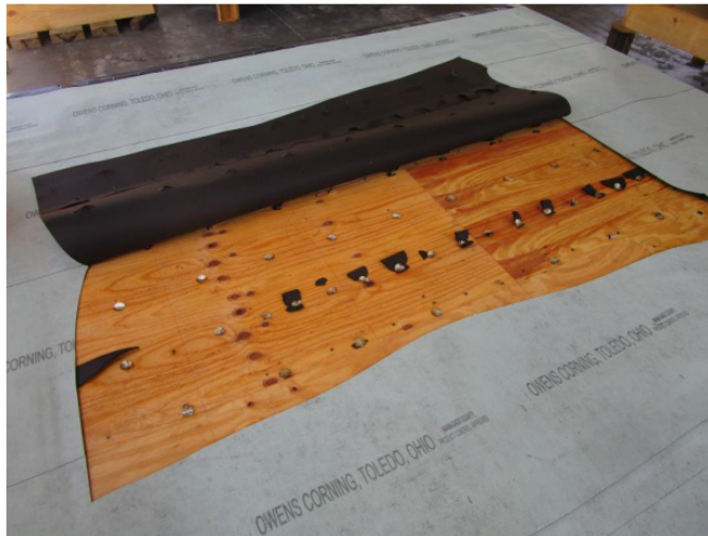
Specimen #4 failure – fastener pull-through
