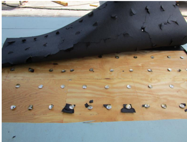
Specimen #2 failure – fastener pull-through
