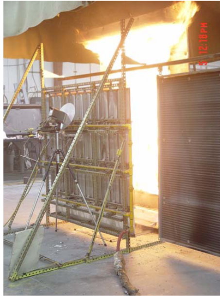
FIGURE 4. IGNITION AND SPREAD OF FLAMES OVER A SPECIMEN.
