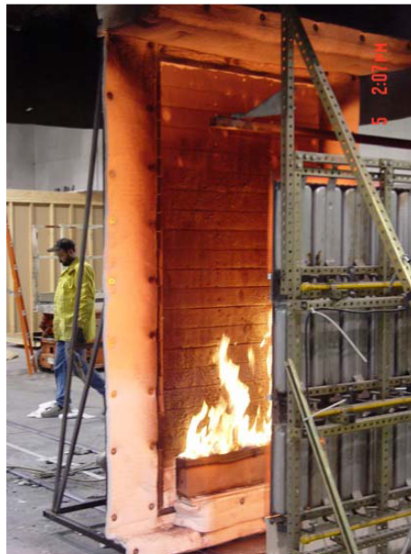
FIGURE 5. SLOT BURNER AT BOTTOM IS IGNITED AFTER 5 MINUTES OF RADIANT FLUX EXPOSURE
