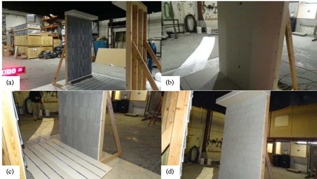
Figure 2. Representative dual-wall systems showing (a) Test 1 burner wall, (b) Test 2 receiver wall, (c) Test 3 receiver wall, and (d) Test 5 receiver wall.
