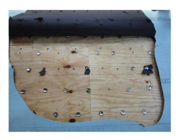
Specimen #5 failure – fastener pull-through
