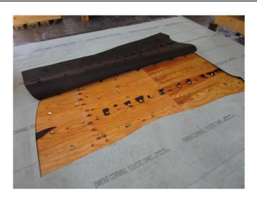
Specimen #4 failure – fastener pull-through
