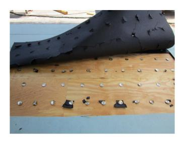
Specimen #2 failure – fastener pull-through
