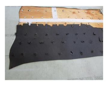
Specimen #3 failure – fastener pull-through
