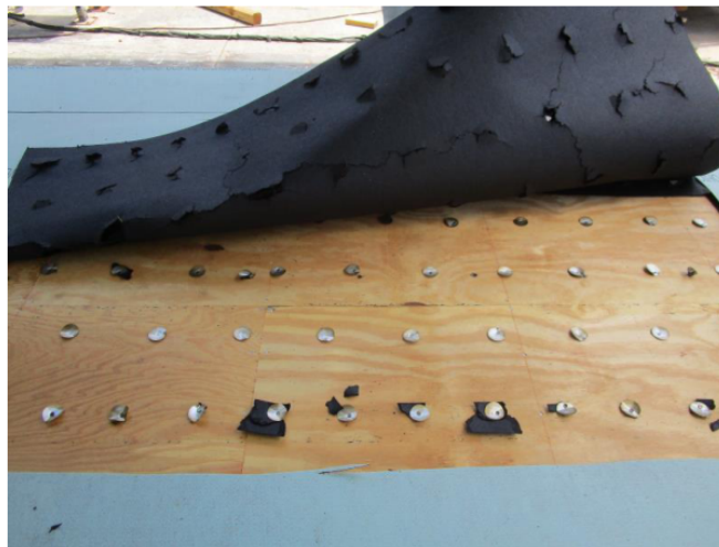
Specimen #2 failure – fastener pull-through
