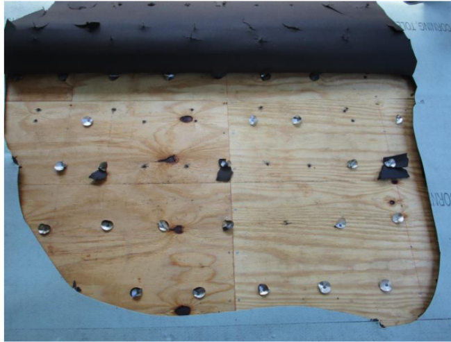
Specimen #5 failure – fastener pull-through
