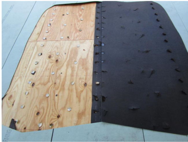
Specimen #1 failure – fastener pull-through
