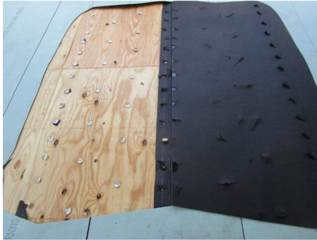
Specimen #1 failure – fastener pull-through
