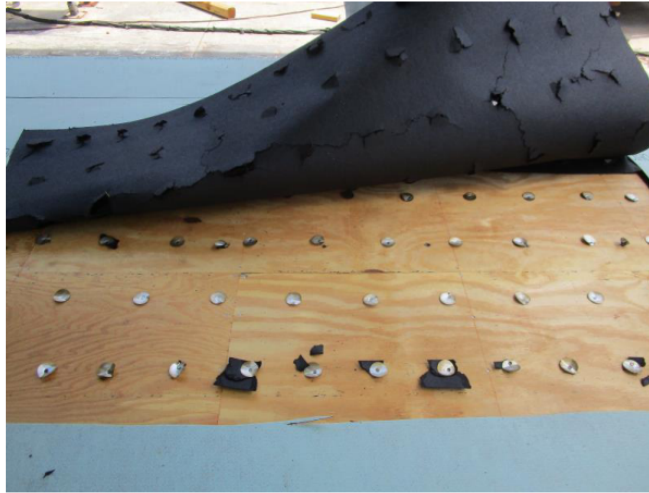
Specimen #2 failure – fastener pull-through
