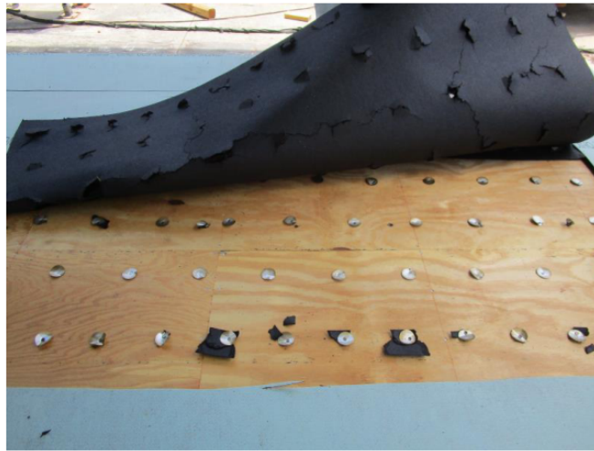
Specimen #2 failure – fastener pull-through
